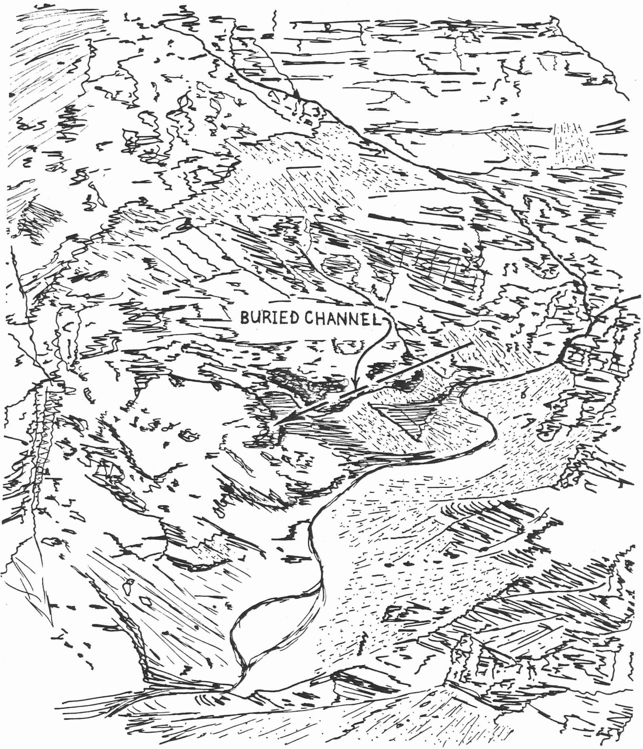
Figure 18 - Illustration of Tapeats Creek Buried Channel
