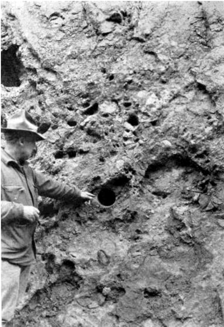
6-inch cores were extracted from the abutments for unconfined compression tests
