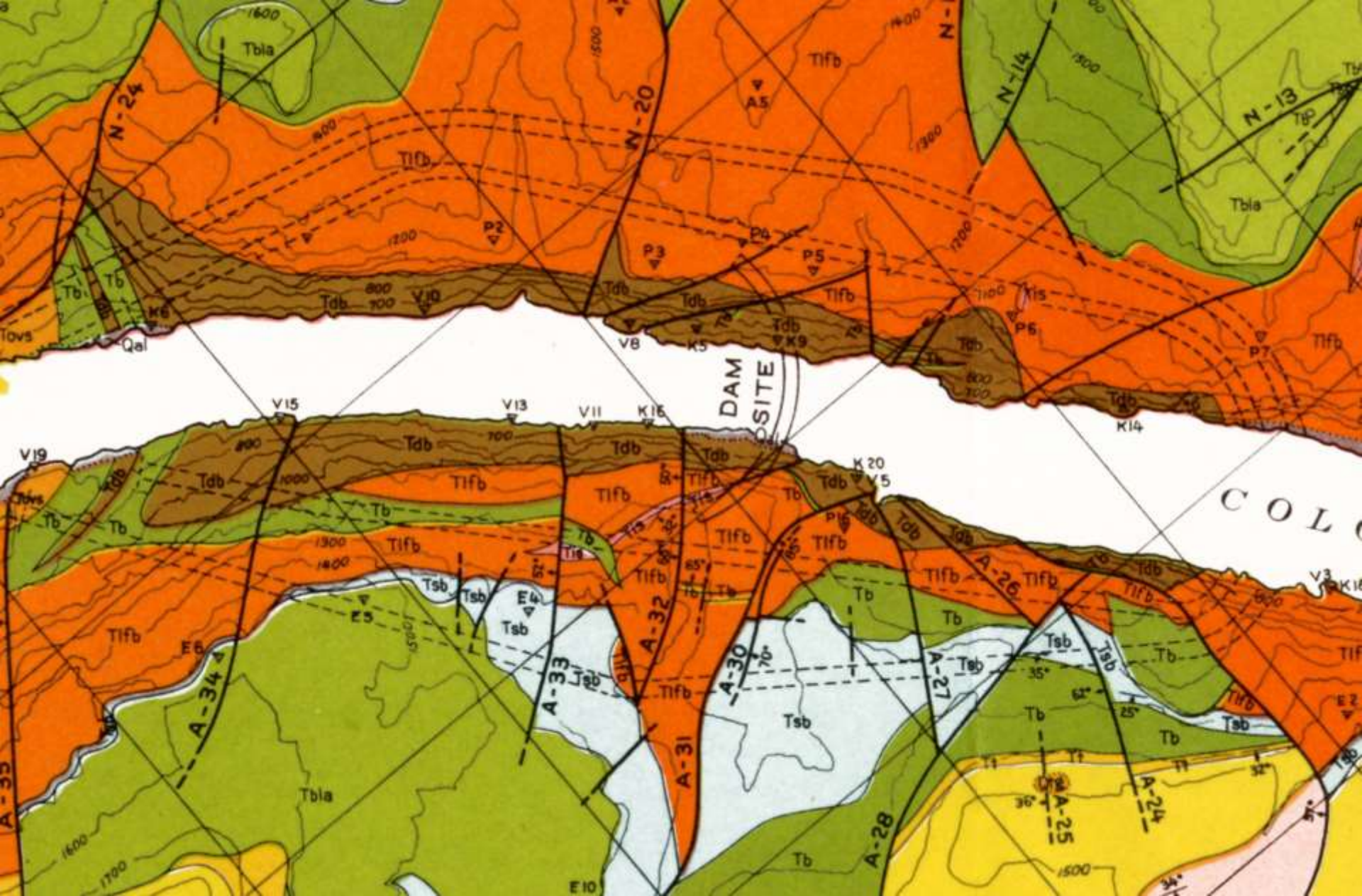
Ransome's geologic map controlled the position of the dam's axis, to wedge the dam in between the two prominent faults mapped on the right abutment
