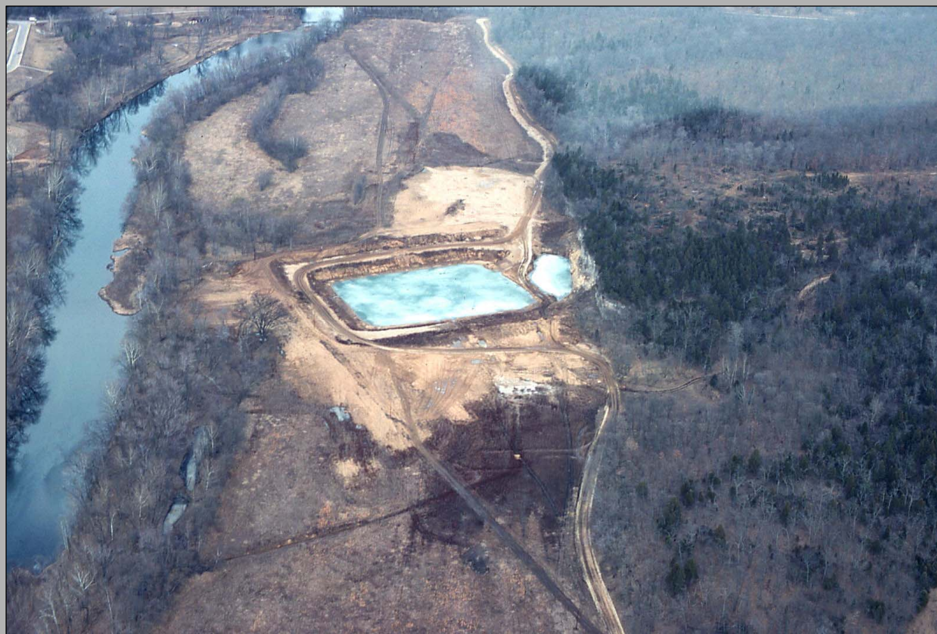
Excavations preparing dam abutments as they appeared in Feb 1977
