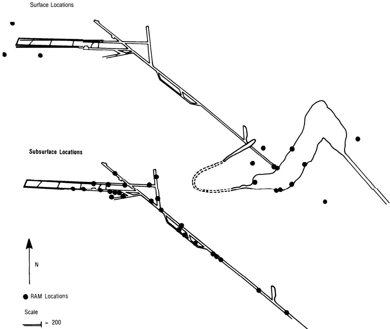
A total of 41 RAMs (15 above the surface, 26 belowground) are used to monitor the containment of radioactive material from a horizontal tunnel test.
