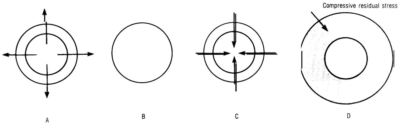
1 ) Cavity expands outward and deforms surrounding rock. 2) Natural resistance to deformation stops expansion. 3) Cavity contracts (rebounds) from elastic unloading of distant rock. 4) Rebound locks in compressive residual stress around cavity.
