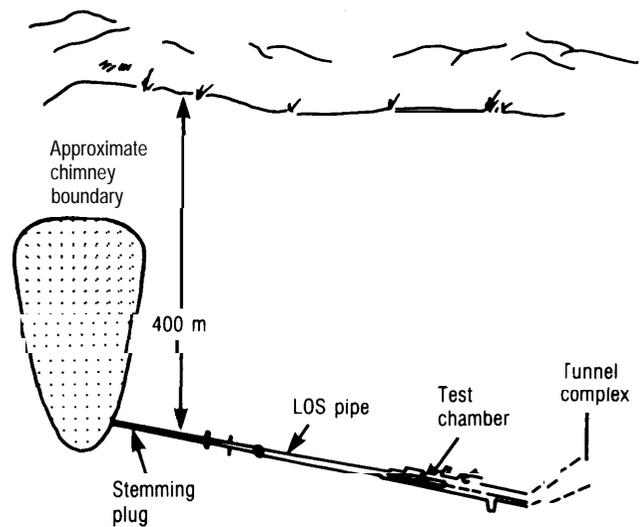
Tunnel shots are typically overburied and the collapse chimney rarely extends to the surface.
