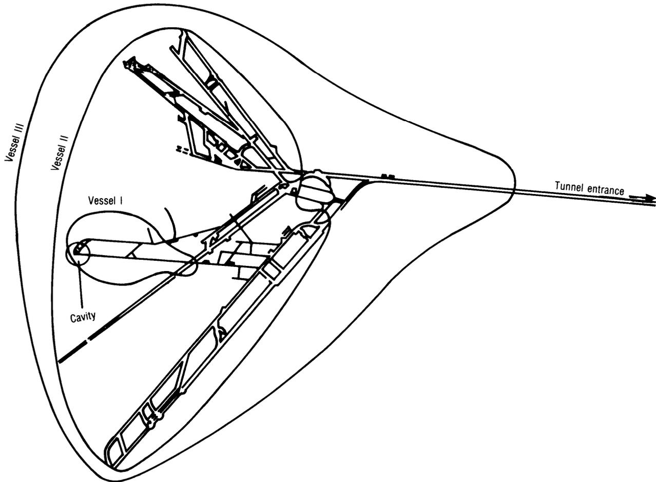
Three containment vessels for the Mighty Oak Test conducted in the T-Tunnel Complex.
