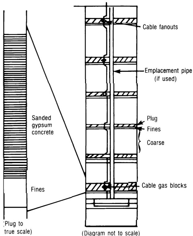
Typical stemming sequence of coarse material, fine material, and sanded gypsum plug used by Lawrence Livermore National Laboratory for vertical drill hole tests.
