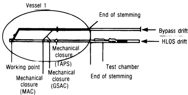
Key: GSAC = gas seal auxiliary closure; MAC = modified auxiliary closure; TAPS = Tunnel and pipe seal
