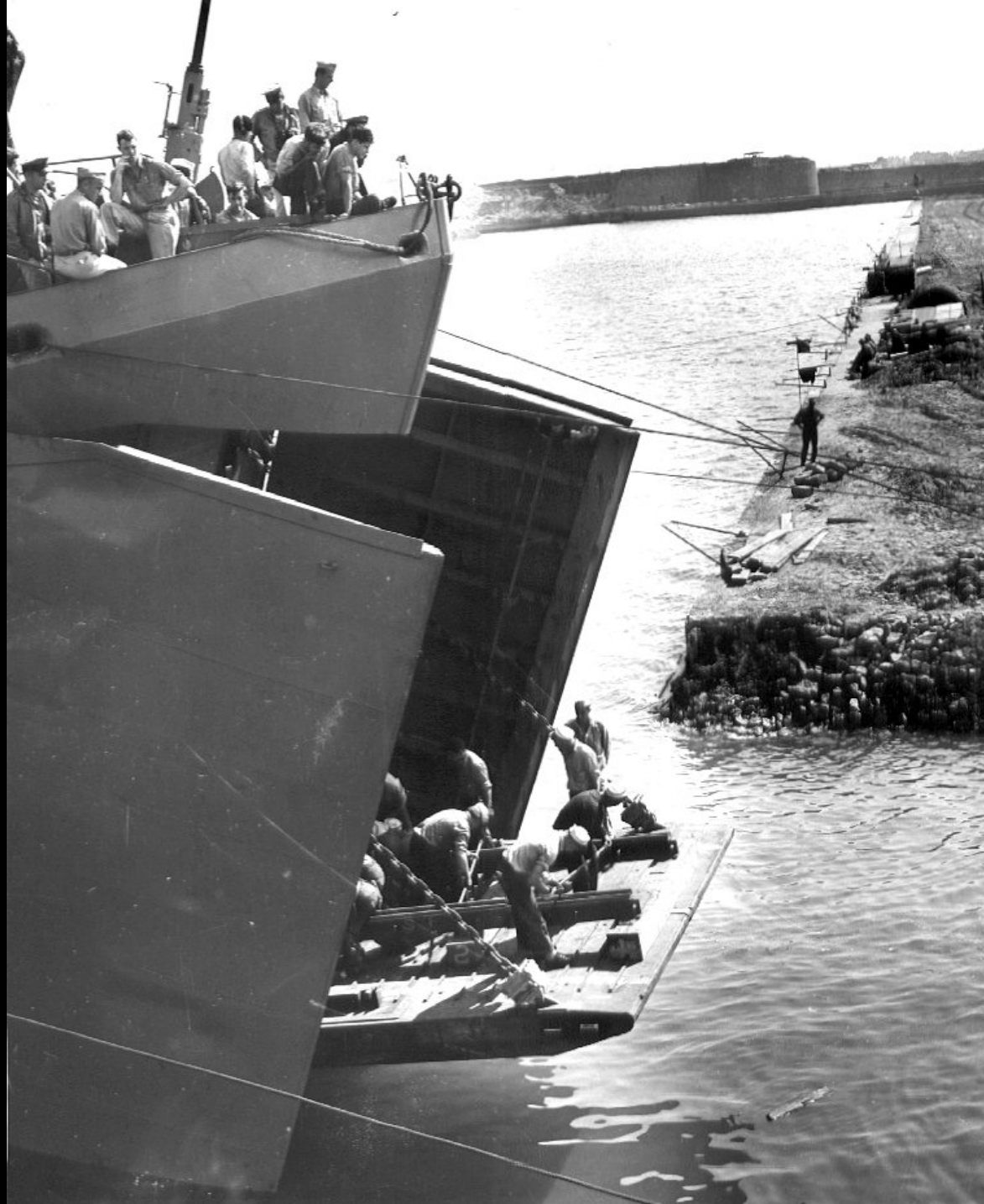
American LST lower bow ramp equipped with rails for unloading railroad rolling stock
