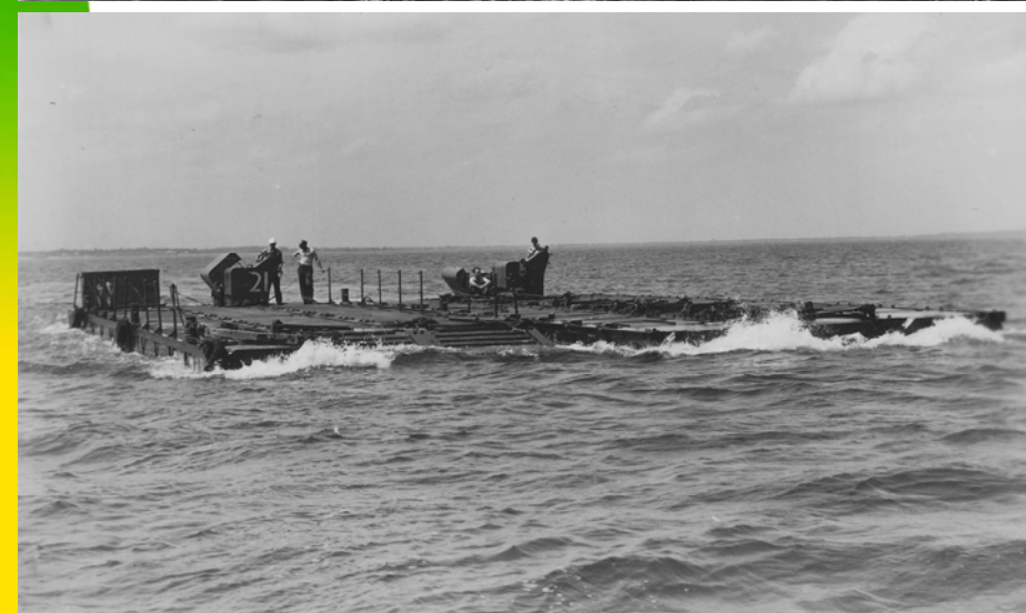
Load tests on two self-propelled 3 x 12 50-ton barges, their maximum capacity
