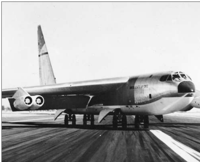
The B-52 was equipped with tandem gear that could be swiveled in to provide crabbing for cross-wind landings
