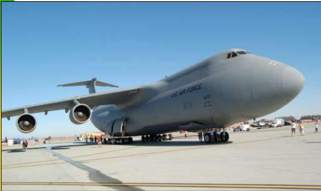
The Lockheed-Martin C-5B Galaxy has a maximum takeoff weight of 769,000 lbs, supported on 32 tires
