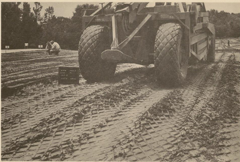
PHOTOGRAPH 8. 20,000-lb wheel load, 12 coverages, 19% water content
