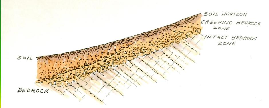
Overexcavation involves removing poor quality foundation materials, such as the soil horizon, colluvium and the bedrock creep zone.
