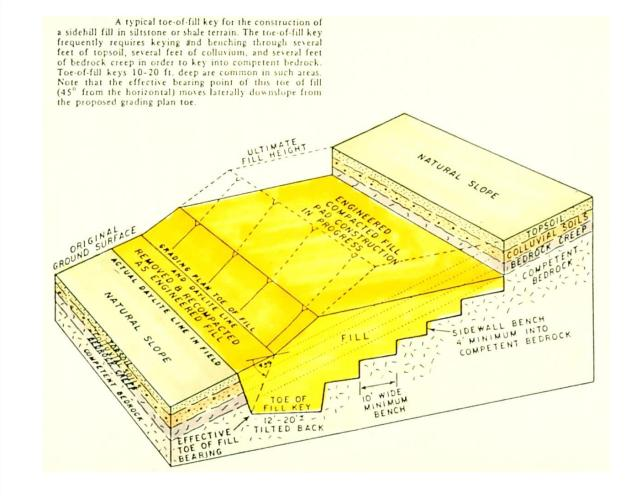
The Modern Grading Code introduced standardized requirements for over-excavation of embankment foundations similar to what had been developed for earthfill dams. This shows Orange County's standard, introduced in 1965.
