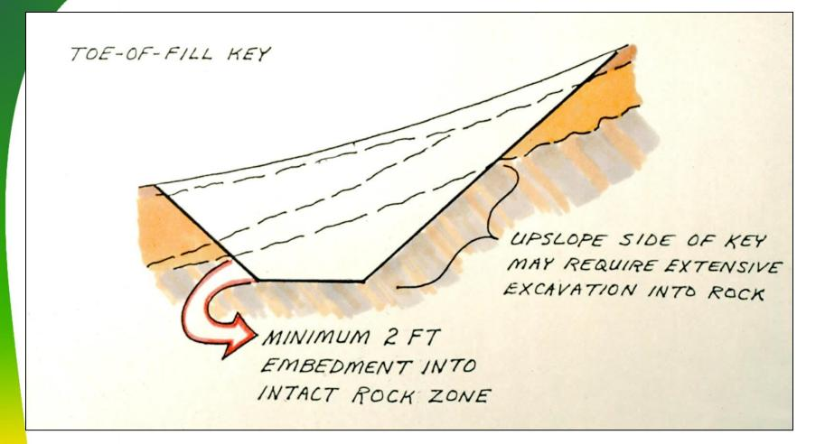
Keyways should extend a minimum of 2 feet into intact foundation materials on the downslope, or frontslope side, of the toe-of-fill keyway, as sketched here.
