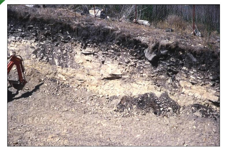
Mapping of the bedrock creep zone is important on sloping ground, especially in expansive soils and slopes floored in siltstone or shale, because this zone serves as a conduit for percolating water.
