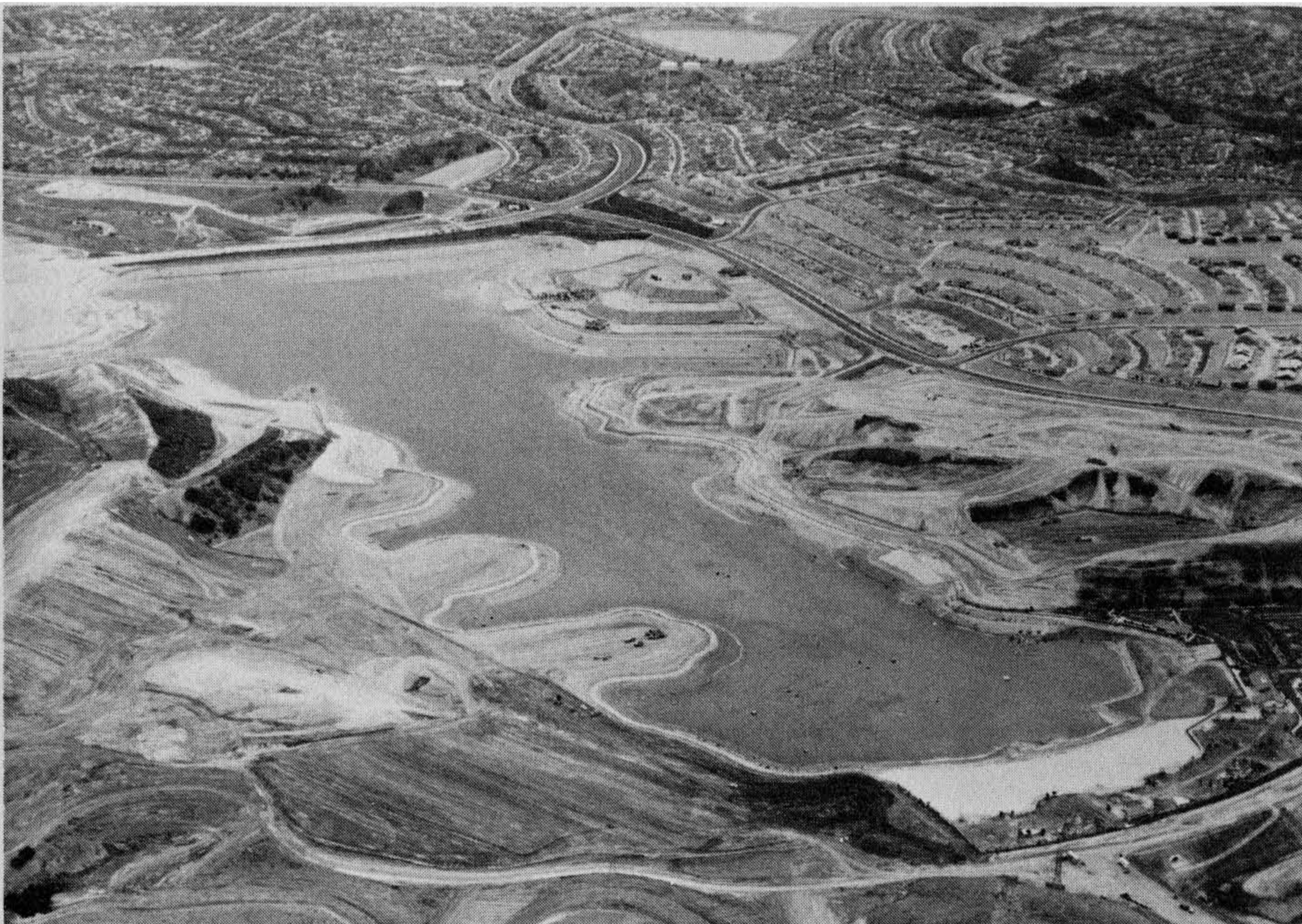
Figure 2.10 Lake Mission Viejo during drought moratorium of lake filling, August 1977. The soil cement and bulkhead edge have been completed, and sand for the main beach is in place. (Lower right). Residential construction is shown in progress at upper right. Photograph by Aerial Eye, Inc., courtesy of the Mission Viejo Company.
