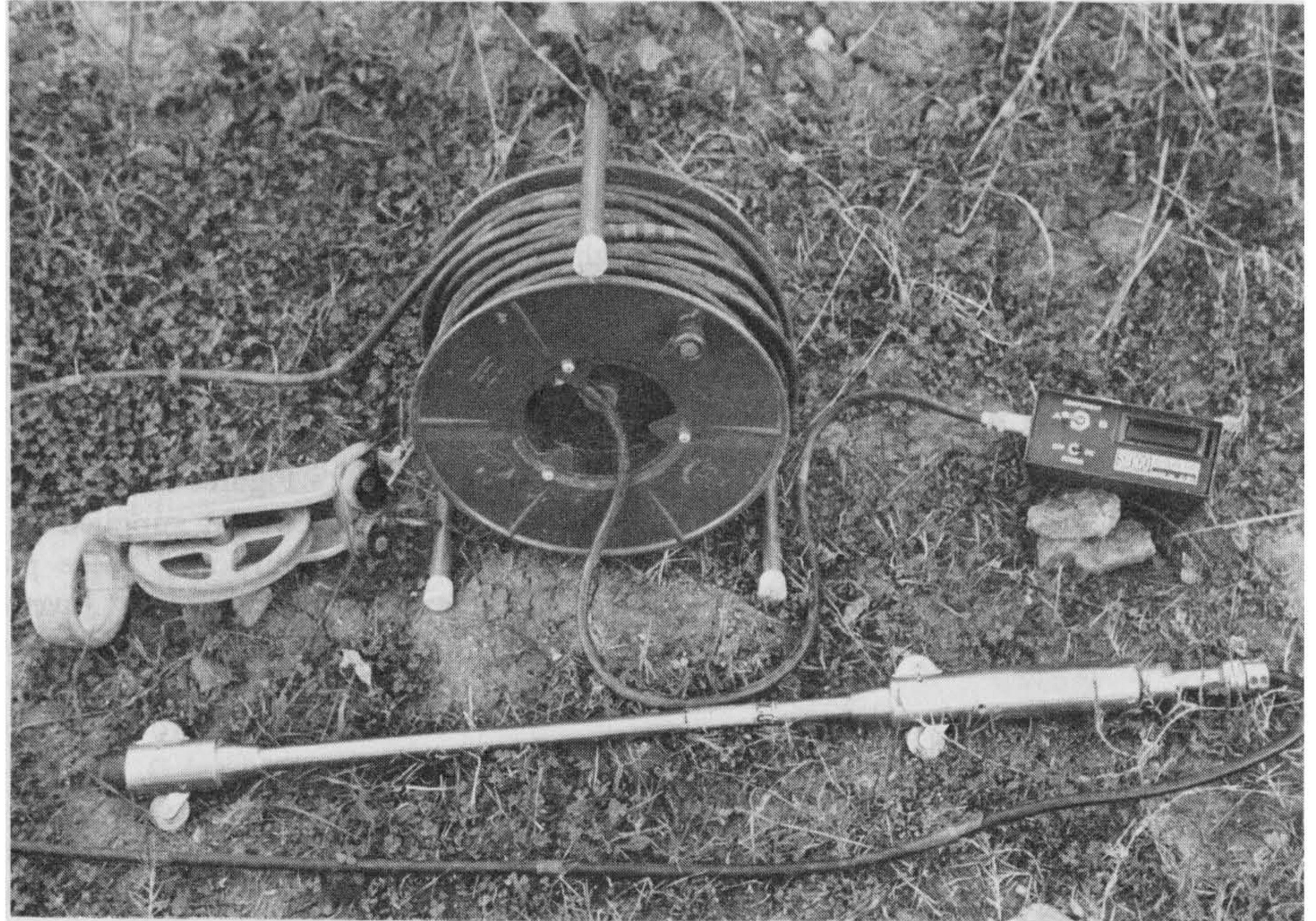
Figure 6-29 (a) Slope indicator inclinometer apparatus is shown, including the inclinometer sensor (foreground), the pulley assembly with cable hold (upper left), cable reel (upper center) and a portable field indicator (right). (b) Operation of the slope indicator inclinometer is shown. James L. Glaze, geologist (left), lowers the sensor with the pulley assembly as Delmar D. Yoakum, soil engineer, reads and records the field data. Photographs by and courtesy of Delmar D. Yoakum, GeoSoils, Inc.
