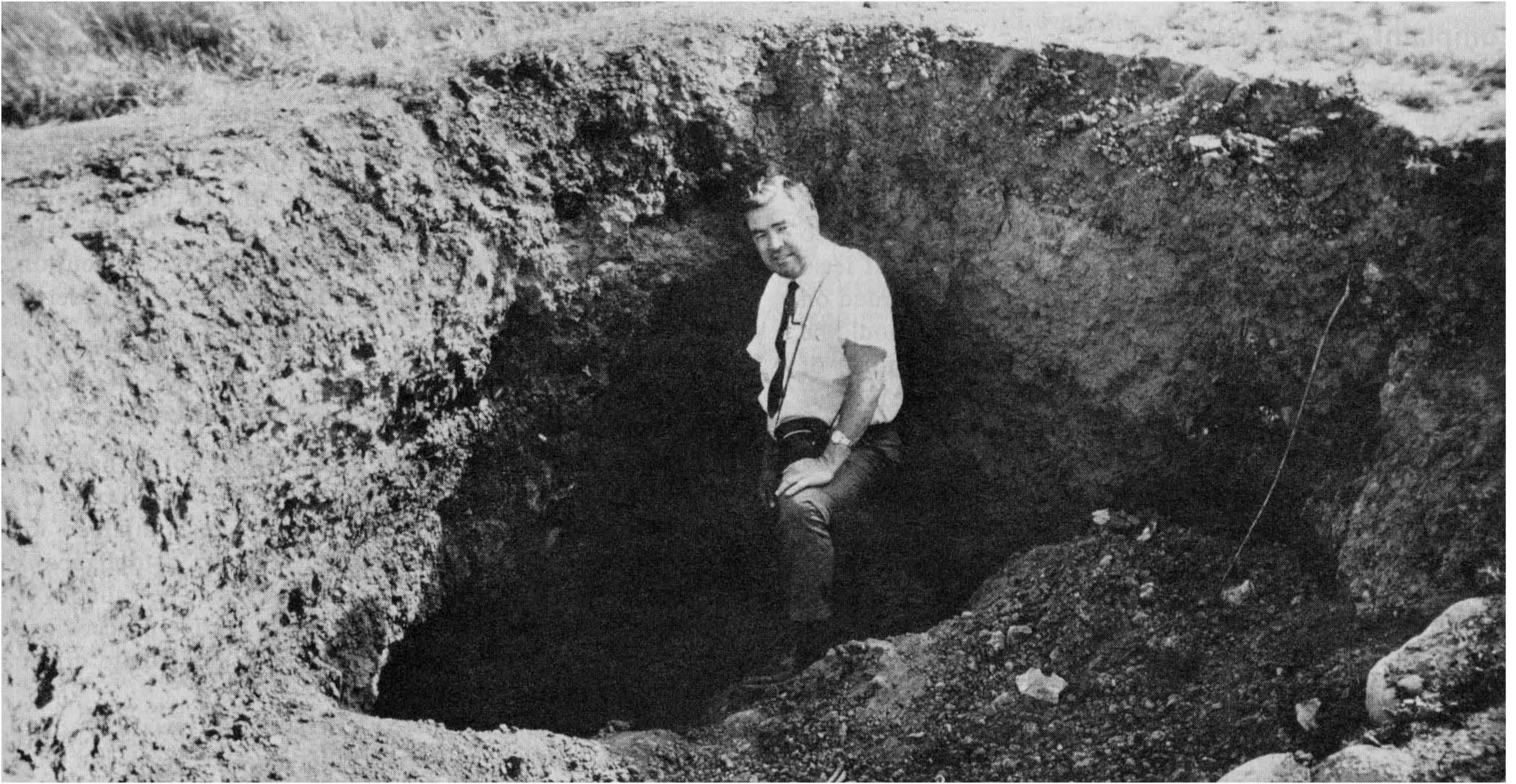
Figure 6-45 Robert W. Ross, supervising grading inspector, County of Orange, CA, stands in a collapsed piping tunnel. This type of collapse is caused by water flow into gopher holes that carried the water down into joints and fractures and pipe out at lower elevations. The subsequent collapse of the overburden leaves huge cavities and concentrates surface flow. Photograph by C. Michael Scullin.
