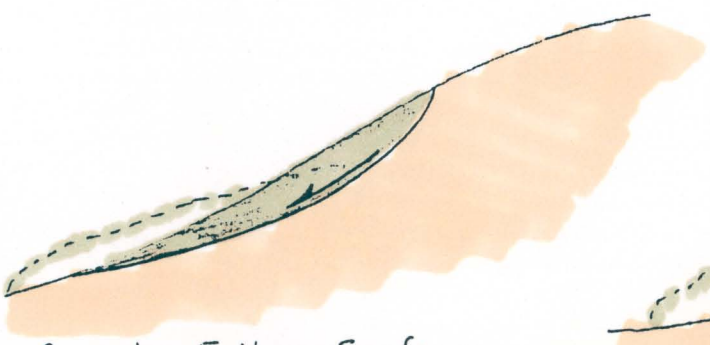
Circular Failure Surfaces in Clays
