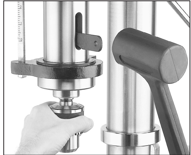
Figure 32. Using drift key to remove arbor.
