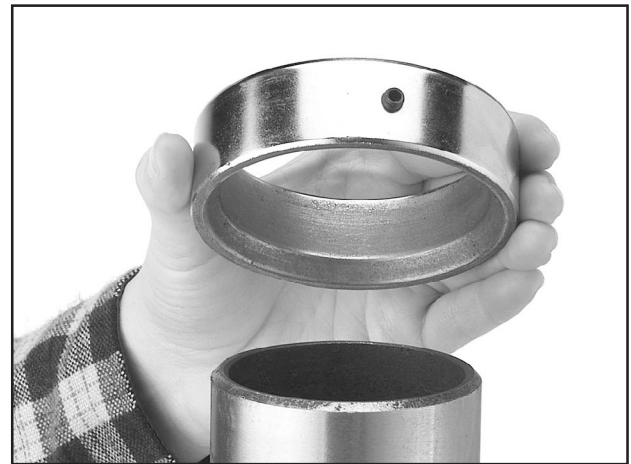
Figure 10. Correct column ring orientation.
