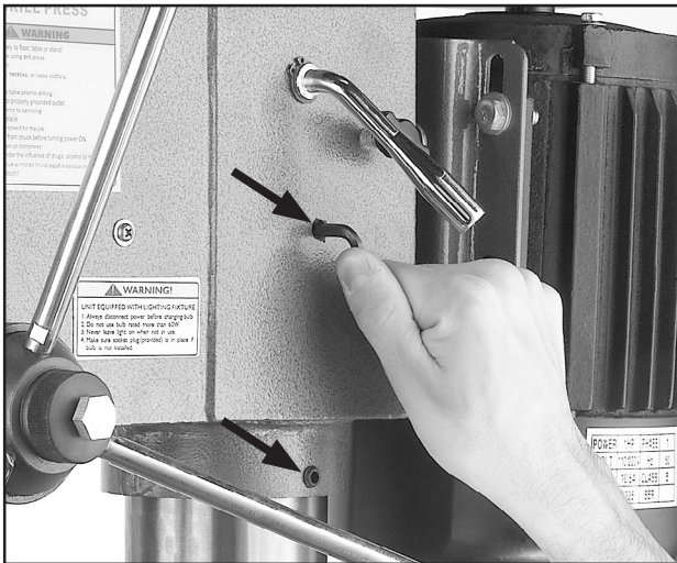
Figure 14. Securing headstock to column.
