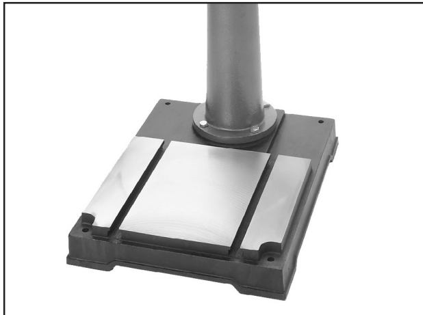
Figure 6. Column secured to base.
