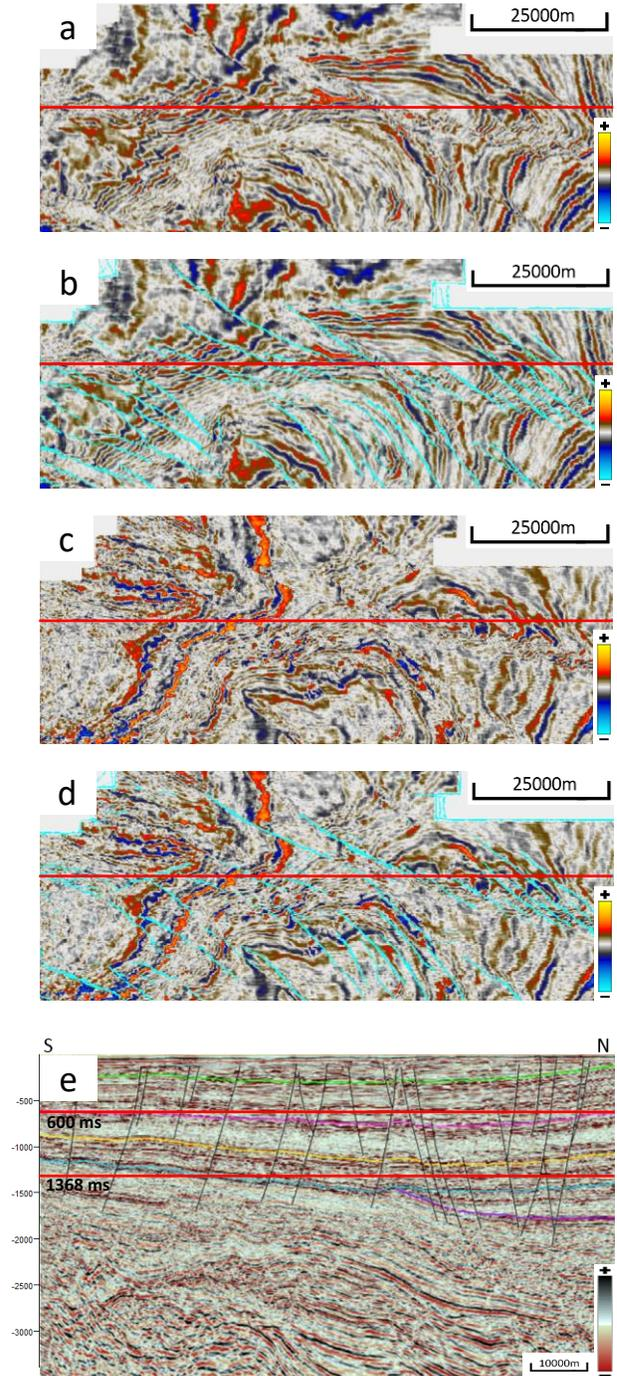
Figure 7. (a) Time slice at 600 ms. (b) Combined ant tracking with seismic volume. (c) Time slice at 1368 ms. (d) Combined ant tracking with seismic volume. (e) Vertical section of inline 665.
