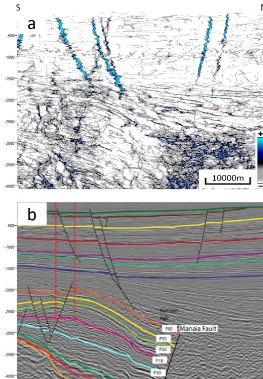
Figure 6. Comparison of the ant tracking result and the conventional fault interpretation. (a) Ant tracking map of inline 692. (b) Conventional fault interpretation of the same inline (Sykes, 2012).
