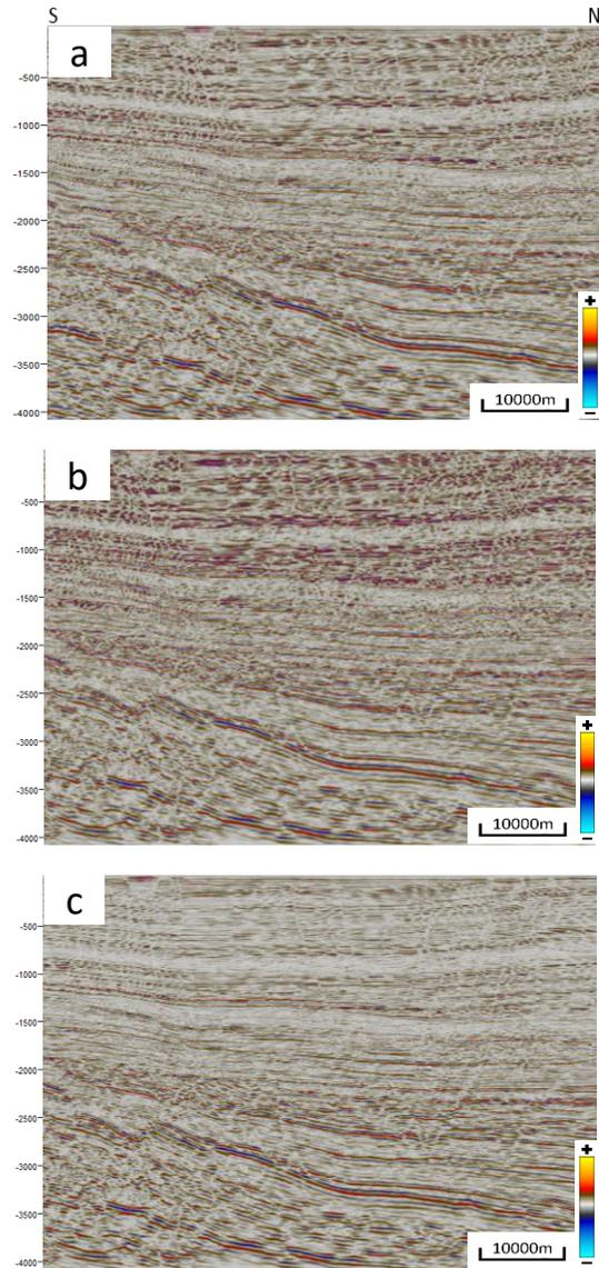
Figure 4. Comparison of the original and processed data of inline 585. (a) Original seismic section. (b) Resulting section after increasing the amplitude of frequency band between 40 and 80 Hz. (c) Resulting section after decreasing the amplitude of frequency band between 40 and 80 Hz.
