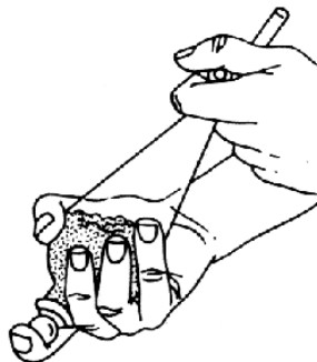
Figure 2: Inverting a separatory funnel.
