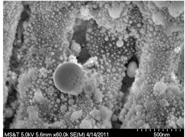
Fig. 3. SEM image of the silicon substrate after fs laser machining, gold coating, and ns laser melting.
