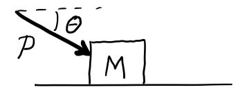
Derive expressions for the acceleration of the crate and the magnitude of the normal force acting on the crate, in terms of relevant system parameters.
