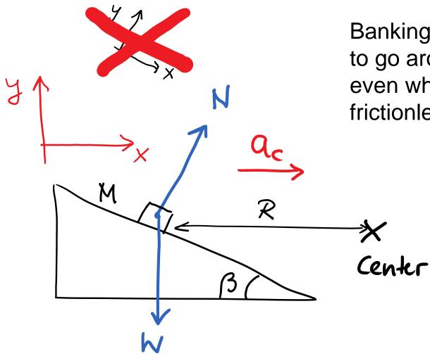
Banking makes it possible to go around the curve even when the road is frictionless.
