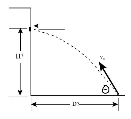
Derive expressions for the horizontal distance *D* he is from the building, and for the height of the window above launch point (i.e. Romeo's hand).
