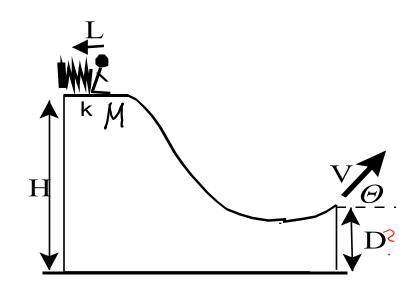
Determine the height *D* of the end of the ski jump in terms of given system parameters.
