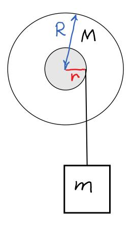
A small disk of radius r is glued onto a large disk of radius R that is mounted on a fixed axle through its center. The combined moment of inertia of the disks is *I*. A string is wrapped around the edge of the small disk, and a box of mass *m* is tied to the end of the string. The string does not slip on the disk. The box is released from rest. Find the speed of the box after it has descended a distance d.
