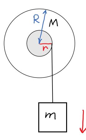
A small disk of radius r is glued onto a large disk of radius R that is mounted on a fixed axle through its center. The combined moment of inertia of the disks is *I*. A string is wrapped around the edge of the small disk, and a box of mass m is tied to the end of the string. The string does not slip on the disk.
