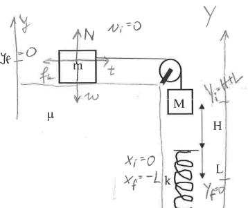
$$\frac{1}{2}(m+M) v_{4}^{2} + mgy_{6}^{2} + Mgy_{6}^{2} + \frac{1}{2} kx_{6}^{2} - \frac{1}{2}(m+M) v_{1}^{2} + mgy_{1}^{2} + Mg y_{1}^{2} + \frac{1}{2} kx_{6}^{2} = Mg(m+M) v_{6}^{2} + \frac{1}{2} k(-L)^{2} - Mg(m+L) = \mu N(m+L) \cos 180^{\circ}$$
