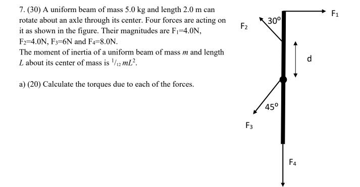
b) (10) Calculate the angular acceleration of the beam. Is it clockwise or counter-clockwise?
