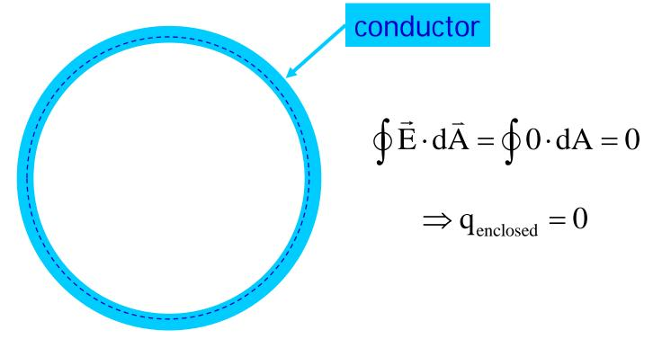
Construct a Gaussian surface that includes the inner surface of the conductor. The electric field at the Gaussian surface is zero, so no electric flux passes through the Gaussian surface. Gauss' Law says the charge inside must be zero. **Any excess charge must lie on the outer surface!** The conductor does not have to be symmetric, as shown.
