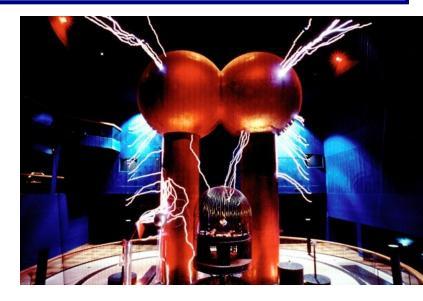
The magnitude of the electric field just outside a charged conductor is equal to  $|\sigma|/\epsilon_0$ , where  $|\sigma|$  is the magnitude of the local surface charge density.
