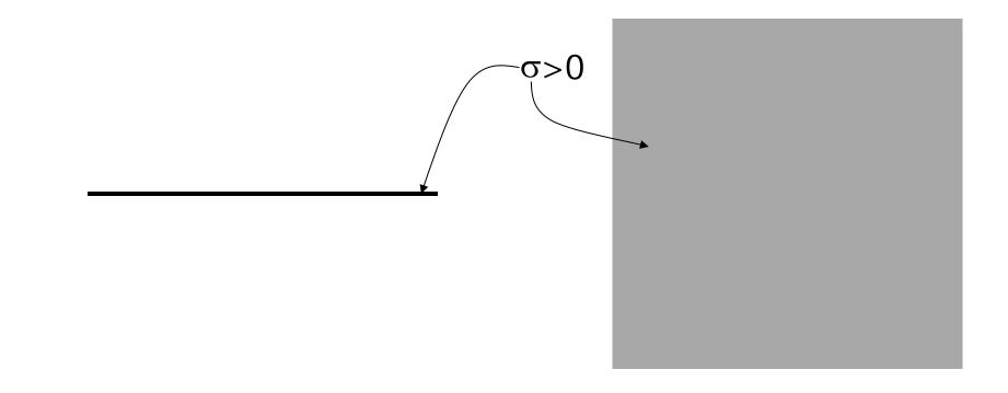
Two views of sheet of charge; side view looking edge on, and top view looking down. Sheet extends infinitely far in two dimensions.
