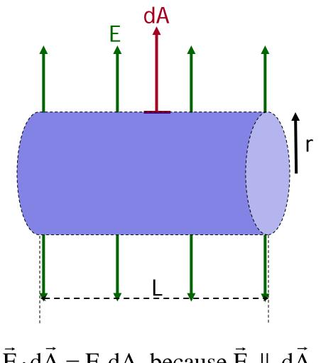
$\vec{E} \cdot d\vec{A} = E dA$  because  $\vec{E} \parallel d\vec{A}$ Also  $\left| \vec{E} \right| = E$  must be constant at any given r.
