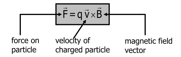
What is the magnetic force if the charged particle is at rest?
