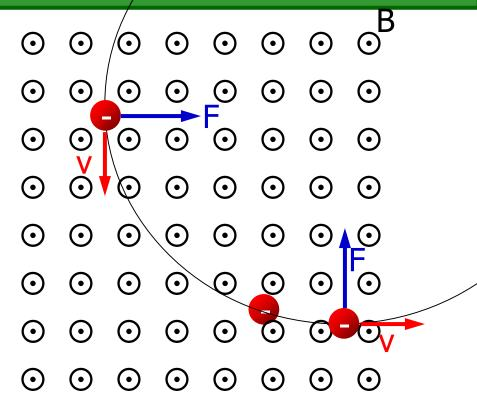
Electron will move in a circular path with a constant speed and acceleration =  $v^2/r$ , where r is the radius of the circle.
