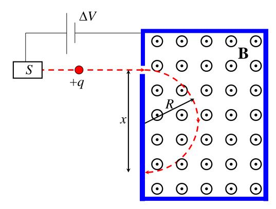
Example: ions from source S enter a region of uniform magnetic field B that is perpendicular to the ion path. The ions follow a semicircle and strike the detector plate at x = 1.7558 m from the point where they entered the field. If the ions have a charge of  $1.6022 \times 10^{-19}$  C, the magnetic field has a magnitude of B = 80.0 mT, and the accelerating potential is  $\Delta V = 1000.0$  V, what is the mass of the ion?
