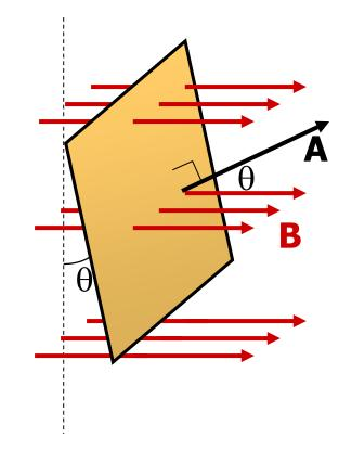
The "amount of surface" perpendicular to magnetic field is  $A\cos\theta$ .
