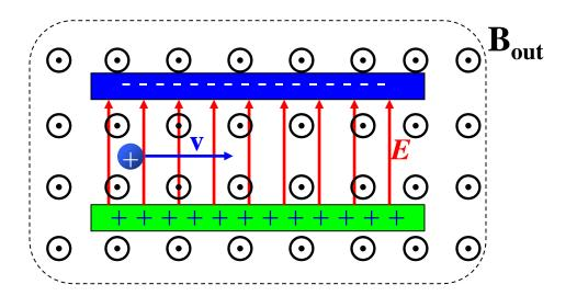
The magnetic field is uniform inside the dashed-line region. What speed will allow the proton to pass undeflected through region of uniform electric field?
