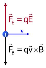
This only works if the electric and magnetic fields are perpendicular and oriented so that  $q\vec{v} \times \vec{B}$  is antiparallel to  $\vec{E}$ .
