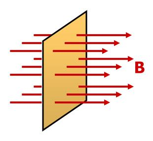
magnetic flux passing through a surface is (proportional to) number of magnetic field lines that pass through it
