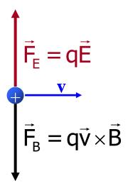
When the electric and magnetic forces balance then the charge will pass straight through.
