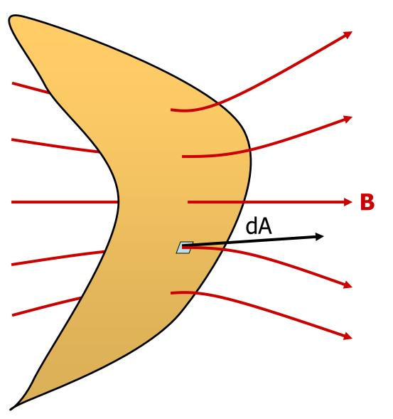
divide surface into infinitesimal surface elements and add flux through each...
