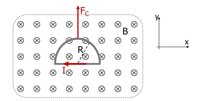
We calculated the force on the semicircular part in the previous example (current is flowing in the same direction there as before).  $F_c = 2 I R B$
