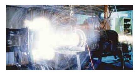
Current in the rails (perhaps millions of amps) gives rise to magnetic field (we will study this after exam 2). Projectile is a conductor making contact with both rails. Magnetic field of rails exerts force on current-carrying projectile.
