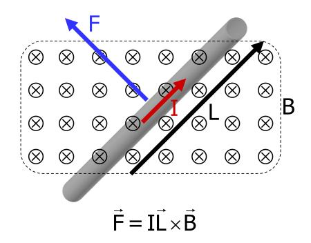
Valid for straight wire, length L inside region of magnetic field, constant magnetic field, constant current I
