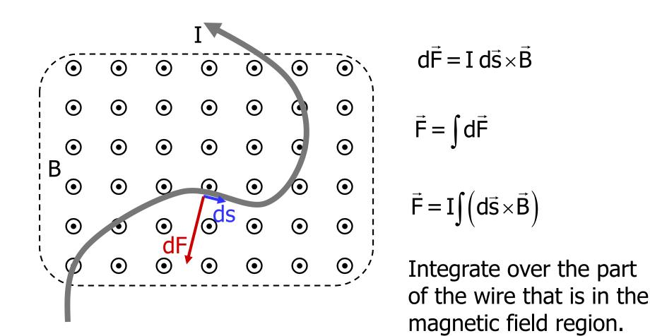
Homework Hint: if you have a tiny piece of a wire, just calculate dF; no need to integrate.
