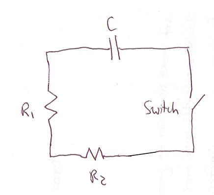
In the circuit shown  $R_1$ =5.0 k $\Omega$ ,  $R_2$ =10 k $\Omega$ , and V = 12.0 V. The capacitor is allowed to fully charge and the battery removed from the circuit. How long does it take for the voltage across the capacitor to drop to  $\frac{1}{4}$  of its fully-charged value?
