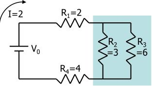
$R_1$ ,  $R_{23}$ , and  $R_4$  are in series.
