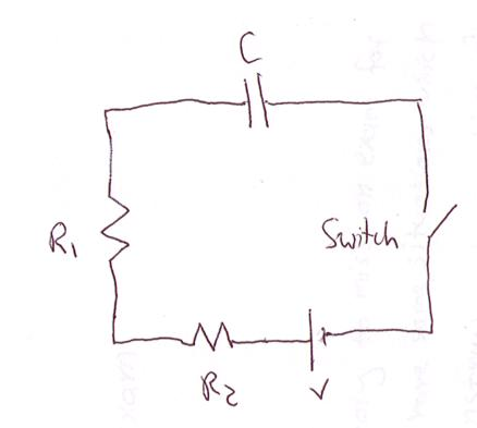
In the circuit shown  $R_1=5.0 \text{ k}\Omega$ ,  $R_2=10 \text{ k}\Omega$ , and V = 12.0 V. The capacitor is initially uncharged. (c) Sketch the current, charge, and potential difference across the capacitor as a function of time.
