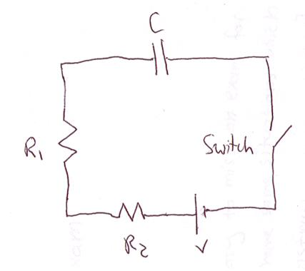
In the circuit shown  $R_1=5.0 \text{ k}\Omega$ ,  $R_2=10 \text{ k}\Omega$ , and V = 12.0 V. The capacitor is initially uncharged. After the switch has been closed for 1.30 µs the potential difference across the capacitor is 5.0 V. (b) Find the value of C.
