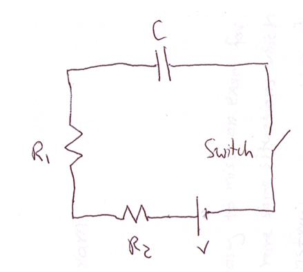
In the circuit shown  $R_1=5.0 \text{ k}\Omega$ ,  $R_2=10 \text{ k}\Omega$ , and V = 12.0 V. The capacitor is initially uncharged. After the switch has been closed for 1.30 µs the potential difference across the capacitor is 5.0 V. (a) Calculate the time constant of the circuit..
