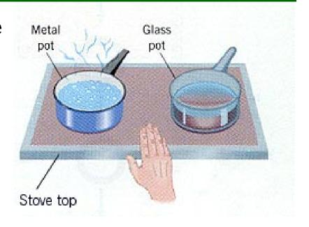
Because the pan has resistance, the current heats the pan. If the coil in the stove has low resistance it doesn't get hot but the pan does.
