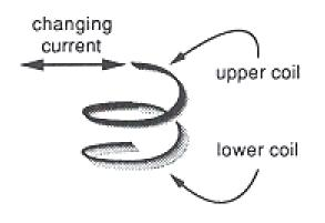
Changing current in upper coil creates a changing magnetic field that induces a counter EMF in the lower coil in a direction to oppose the change of current.
