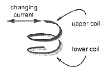
Changing current in upper coil creates a changing magnetic field that induces a counter EMF in the lower coil in a direction to oppose the change of current. The effect is "like" that of friction.
