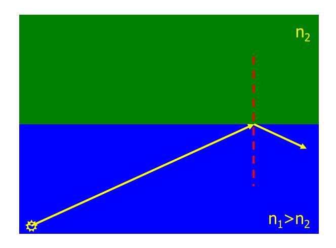
Light incident at any angle beyond  $\theta_{\text{C}}$  is totally internally reflected.
