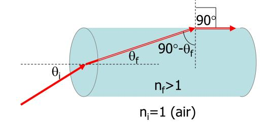
At the critical angle, instead of exiting the fiber, the refracted light travels along the fiber-air boundary. In this case,  $90^{\circ}$ - $\theta_f$  is the critical angle.
