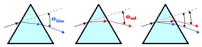
Blue light refracts more than red light due to the difference in wavelength. This causes blue light to deviate from its original path by a greater angle than the red light.
