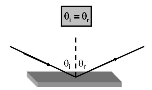
Real Important Note: the angles are measured relative to the surface normal.
