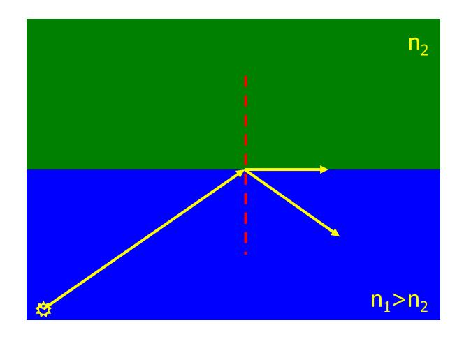
Increasing angle of incidence...more...critical angle reached... some of incident energy is reflected, some is "transmitted along the boundary layer.
