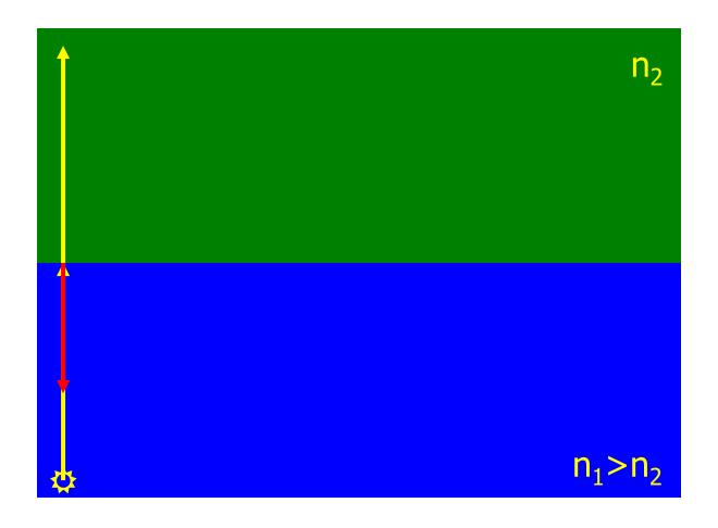
Ray incident normal to surface is not "bent." Some is reflected, some is transmitted.
