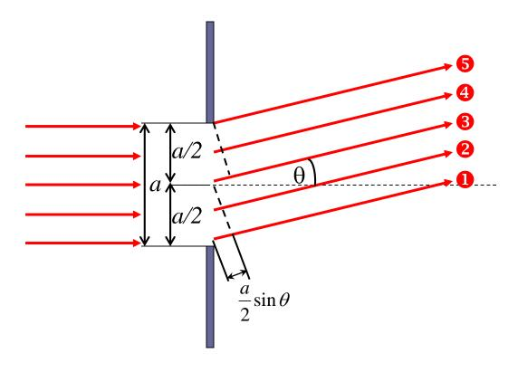
If you divide the slit into 4 equal parts, destructive interference occurs when  $sin\theta = \frac{2\lambda}{a}$ .
