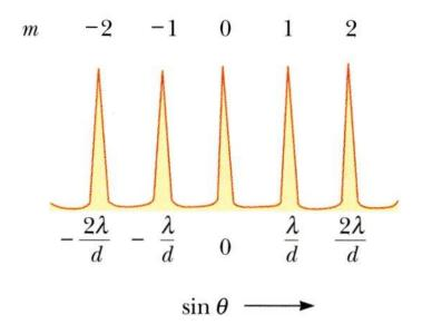
The intensity maxima are brighter and sharper than for the two slit case. See <a href="here">here</a> and <a href="here">here</a>.
