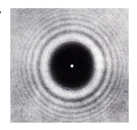
The central bright spot is a result of light "bending" around the edges of the penny and interfering constructively in the exact center of the shadow.
