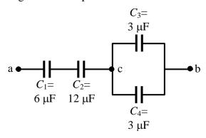
(b) (15 points) Calculate the charge stored in each of the 3 microfarad capacitors ( $C_3$  and  $C_4$ ).
