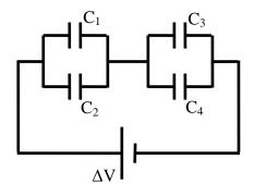
The potential difference  $\Delta V$  applied to this set of capacitors is 10 V. Determine the potential difference across each capacitor and the charge on each. Show your work and put your answers (including units) in the boxes provided.
