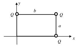
b) Determine the electrical potential at the origin due to these three point charges, assuming that the potential is zero at a point infinitely far away. Express your answer in terms of Q, a, b, and Coulomb's constant k, all of which you should leave in symbolic form. (10 points)
