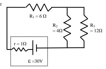
(b) (30 points) Find the voltage across each of the external resistors  $R_1$ ,  $R_2$ , and  $R_3$ , and the current flowing through each of the external resistors  $R_1$ ,  $R_2$ , and  $R_3$ .
