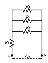
(b) (20 points) The power dissipated in resistor  $R_4$  is 36 W. Determine the current through each resistor.
