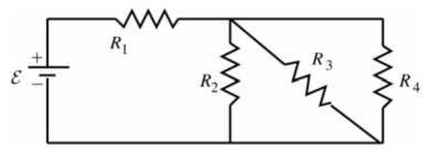
(a) (10 points) Find the equivalent resistance of the resistors connected across the power supply.
