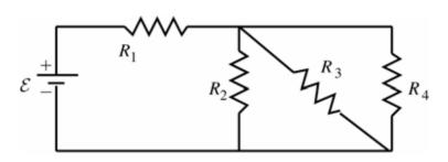
(a) (10 points) Find the equivalent resistance of the resistors connected across the power supply.
