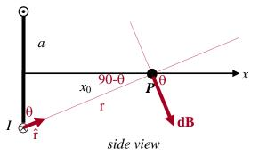
(b) (30 points) Use the Biot-Savart Law to compute  $B_x$ , the *x*-component of the magnetic field at *P*, due to the entire current loop.
