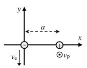
(a) (15 points) Find the magnetic field due to the proton at the position of the electron at the instant shown.
