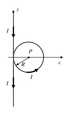
(b) (20 points) Explicitly use the Biot-Savart law to express as an integral the magnetic field  $\vec{B}$  at point P due only to the circular loop of wire. Evaluate your integral and express your result using unit vector notation.
