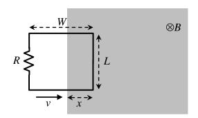
(a) (4 points) Starting with an OSE, derive an expression for the current in the circuit when it has moved a distance *x* into the region of space containing the magnetic field. Then calculate a numerical value for the current.
