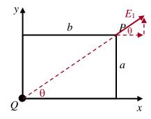
(a) (10 points) Find the x component of the electric field produced by the charge Q at the opposite corner of the rectangle, labeled point P in the diagram.
