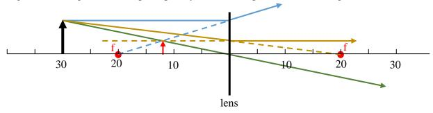
6. (20 points total) An object is placed 15.0 cm away from a converging lens with a focal length of 9.0 cm. (Note: this is not a continuation of problem 5!)
