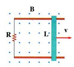
(a) (5 points) What is the direction of the induced emf in the loop formed by the rod, rails and resistor?
