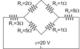
(a) (10 points) Find the equivalent resistance and total current in the circuit.
