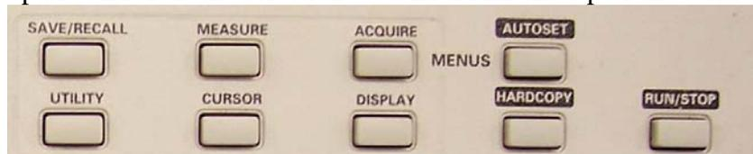
These buttons provide a number of important functions, as well make other menus available. Starting at the far right, the **RUN/STOP** button does exactly what it says. It toggles the acquisition mode between run mode and stop mode.
