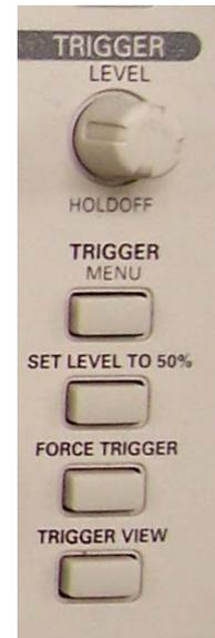
Mentioned in the previous section was a function called **holdoff**. Trigger holdoff sets an amount of time that must elapse before the trigger is re-armed for the next cycle. This value is usually set to 500 nS, which is the fastest that this particular scope can re arm itself.
