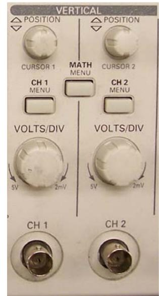
The Menu button activates the selection menu on the right side of the display, and switches its selections to those appropriate for the input channel. For this scope you have the following settings that can be accessed.
