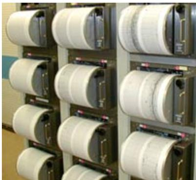
Drum recorders, such as seen at the left, are used to record data over long periods of time. As the drum rotates, the recording needle is indexed slightly to one side, allowing the drum to record for many revolutions. This is typically done when there is only a small amount of data to be recorded, but it may occur at some instant over a long period of time. Drum recorders such as this may record for as long as a week between roll changes.
