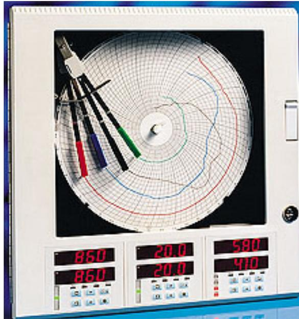
The above two recorders are typical circular recorders. These type recorders are generally set to rotate once every twelve or twenty four hours.
