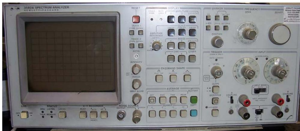
Many people have trouble with the concept of the spectrum analyzer. The simplest model for how one of these systems works, is that there are lots of individual frequency filters. Each filter being set to one specific frequency. If the incoming signal has a component that matches this frequency, the analog voltage level of that component is displayed.
