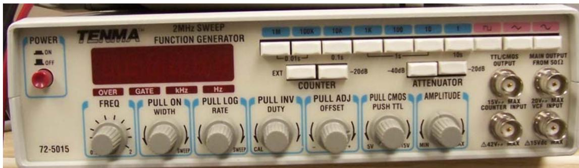
The most important and basic portions of this unit are the frequency control section, the function select section, the amplitude section and the output section.
