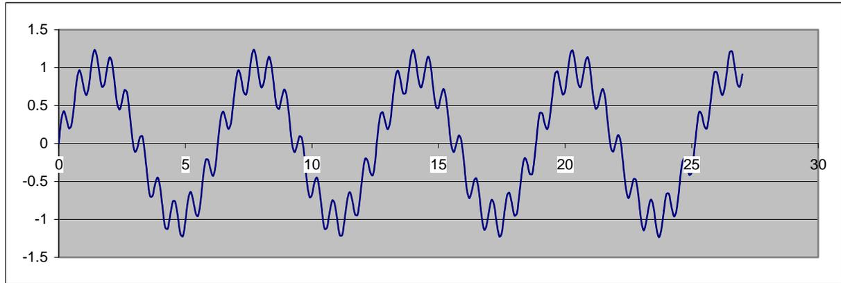
As an example the above waveform contains two sine waves, one at 1 Hz with an amplitude of 2 Volts P-P, and a second component that is 10Hz, with a 0.5V P-P amplitude.
