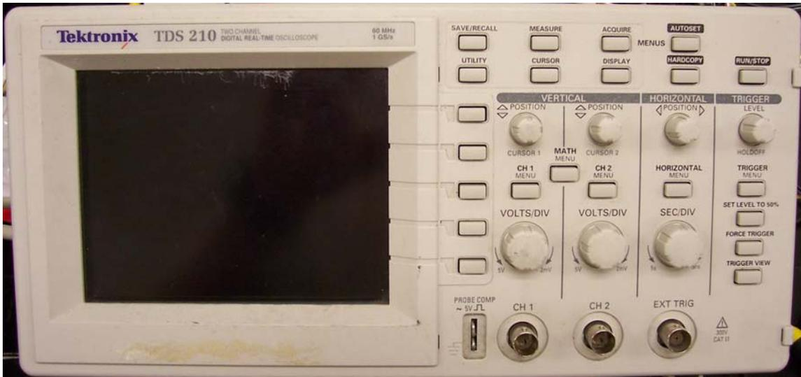
The Tektronix TDS210 used in the lab has vertical deflection controls for each of the two input channels, a horizontal display section controlling the sweep, and a trigger section as described above. In addition to these basic features there are a number of menu driven selections to control measurements and cursors.
