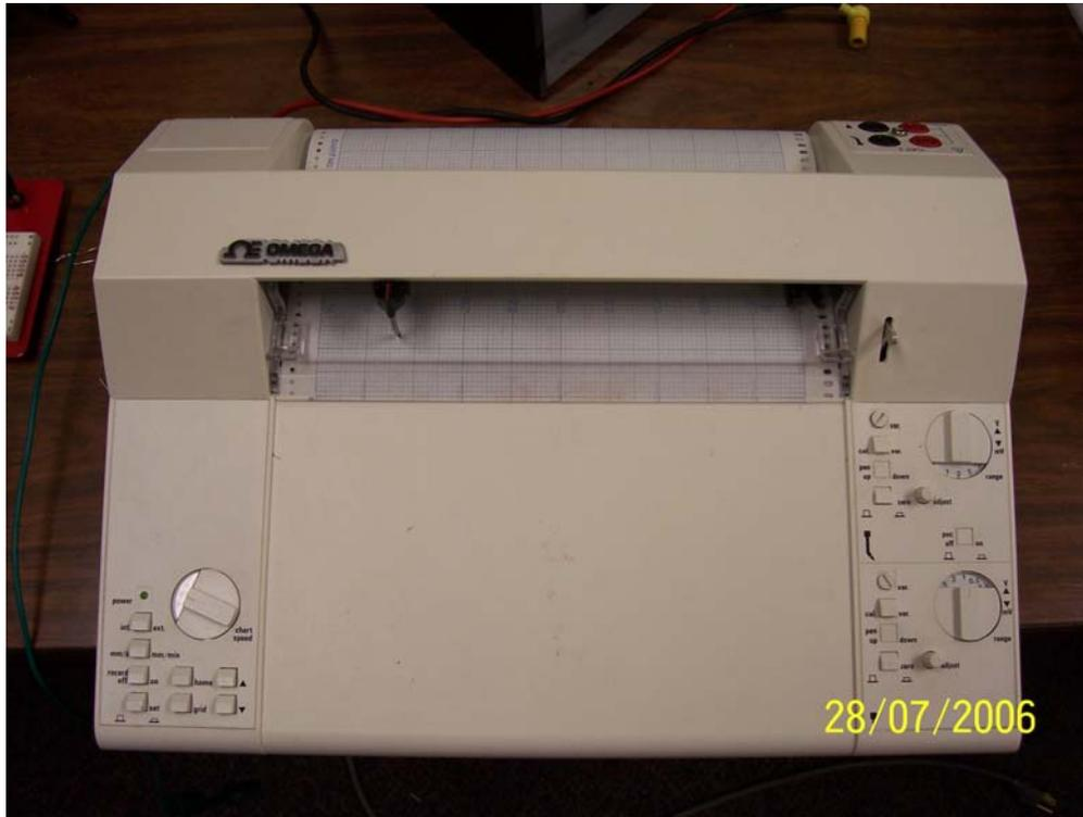
Looking at the lower left of the picture, you can see a set of controls to manage the paper feed. The controls to the right control the motion of two pens.
