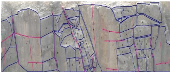
Figure 3.0: Discontinuity map of a rock face. Red lines represent linear traces and blue blocks represent planar facets
