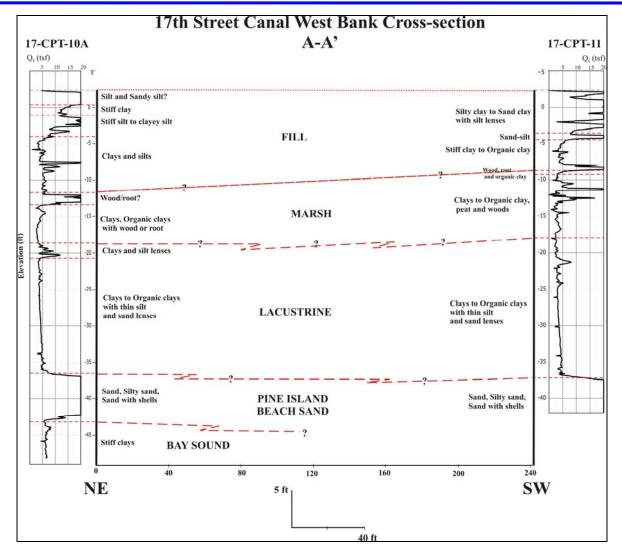
Figure 3.21 - upper: Stratigraphic interpretations between CPT soundings along western embankment of the 17<sup>th</sup> Canal (in Jefferson Parish), opposite the breach on the east side. The marsh-swamp deposits are dipping slightly towards Lake Pontchartrain, while the lacustrine clays appear to be flat lying.
