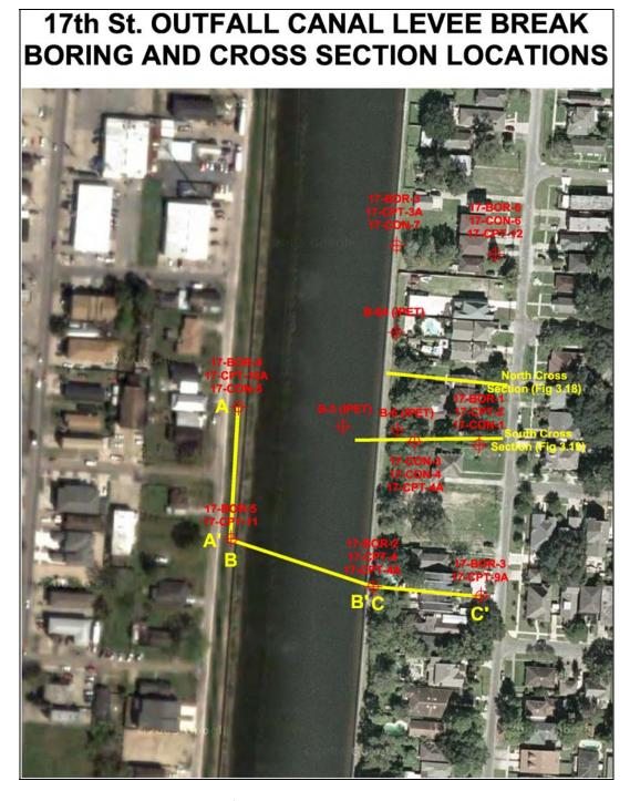
Figure 3.17: Aerial photo of the 17<sup>th</sup> Street Canal breach site before the failure of August 29, 2005. The yellow lines (at middle right) indicate the positions of the geologic sections presented in Figures 3.17 and 3.18, while cross sections A-C' are shown in Figure 3.21.
