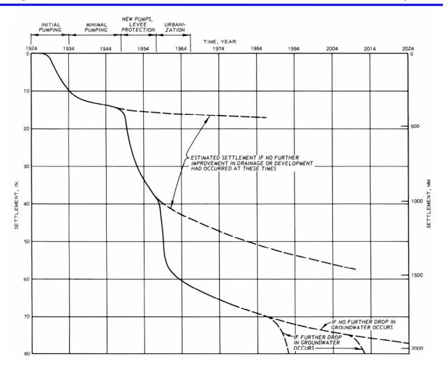
Figure 3.29: Record of historic settlement in the town of Kenner, which is characterized by 6.5 to 8 feet of surficial peaty soils (taken from Kolb and Saucier, 1982). The earlier episodes of settlement were triggered by groundwater withdrawal (for industrial and municipal usage), while the later episode was caused by drainage associated with urban development. This area was covered by dense cypress swamps prior to development.
