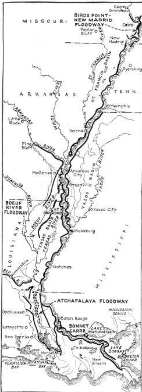
Levee and diversion system of Mississippi flood control adopted by act of Congress approved May 15, 1928
