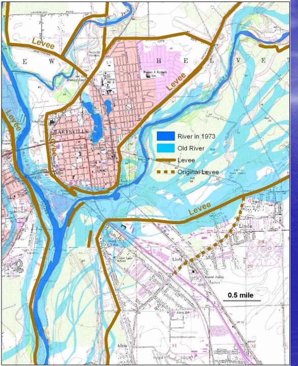
• Taken from updated USGS 7.5 min topographic sheet • The low flow channel had now dropped 20 feet *since 1900*, and was within 6 or 7 feet of its 1849 bed level
