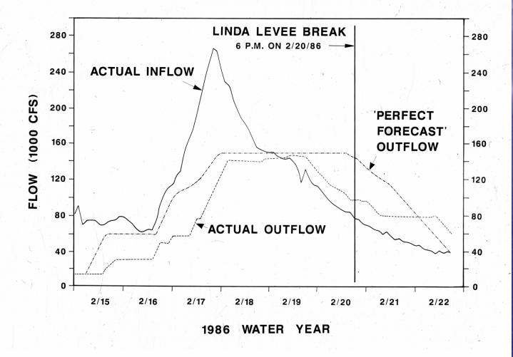
Inflow and discharge from Oroville Reservoir during the February 1986 storm, compared to the forecast outflow by State DWR when the project design was modified, following the December 1964–January 1965 storm sequence.
