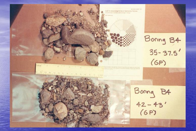
The coarse channel gravels had not been detected in any of the previous geotechnical investigations, not even those FOLLOWING the 1986 levee failure! Ouch!!
