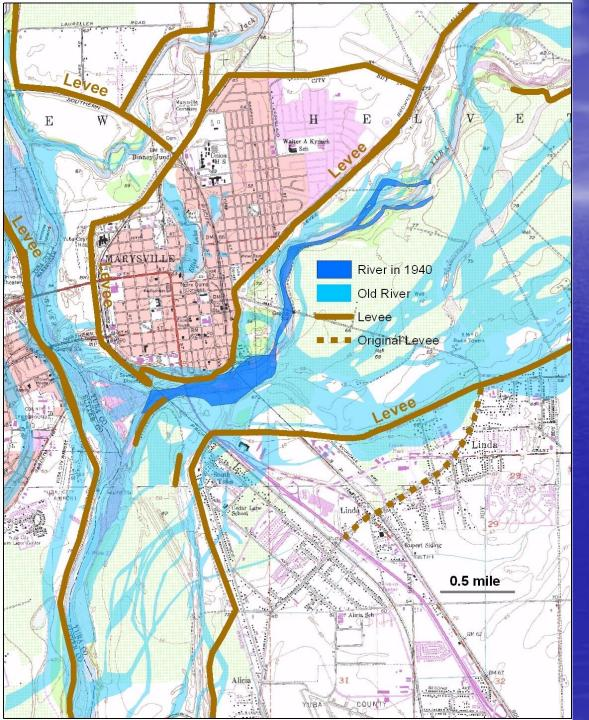
• Taken from a map prepared by the Corps of **Engineers** after the 1940 flood • The attempts to train the main channel were starting to pay off, as the bed had dropped 14 to 16 feet since 1862
