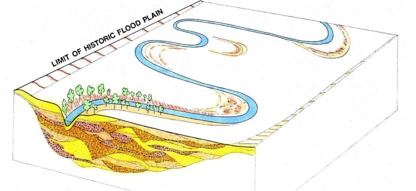
The  $D_{15}$  particle size tends to control permeability; and k can vary by four orders of magnitude in adjacent channel deposits. If you miss the high permeability channels, you fail to characterize the site conditions for any meaningful seepage analyses.
