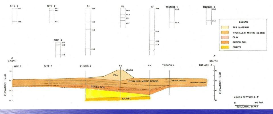
Preliminary Section A-A' cut the levee at 50 degrees to its alignment, along the 'flow path' of the river channel.
