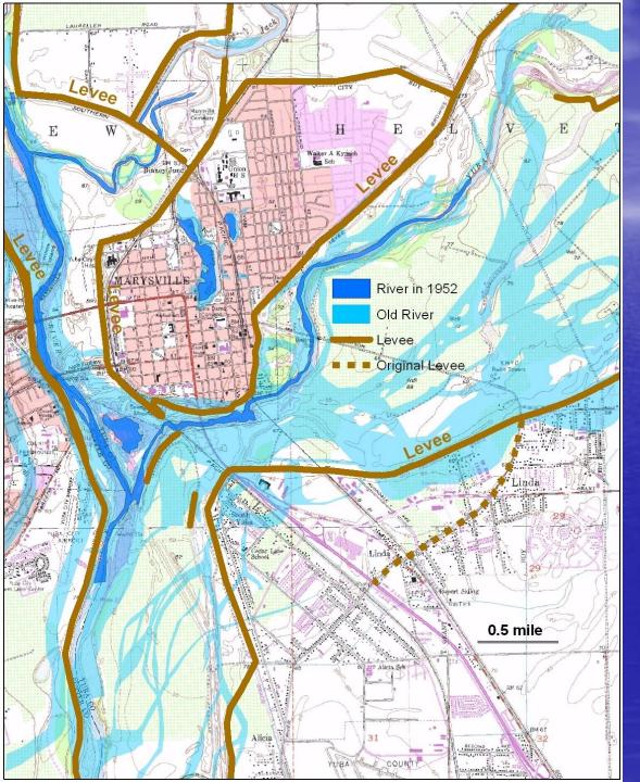
• Taken from first USGS 7.5 min quadrangle The low flow channel is essentially stabilized, incised in the mine slickens and hugging the northern bank.
