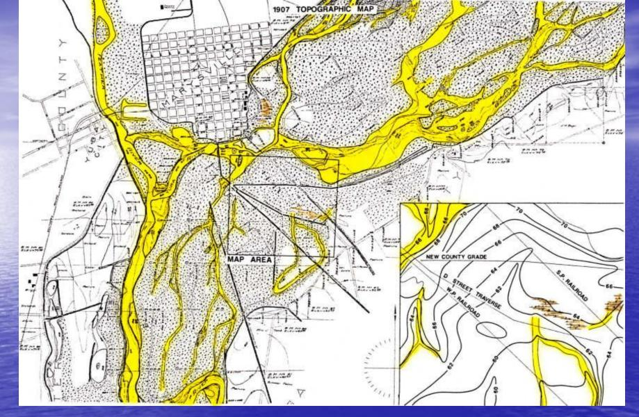
1907 California Debris Commission survey; yellow highlights low flow channels. Insert shows enlargement of the area where the 1986 breach occurred.
