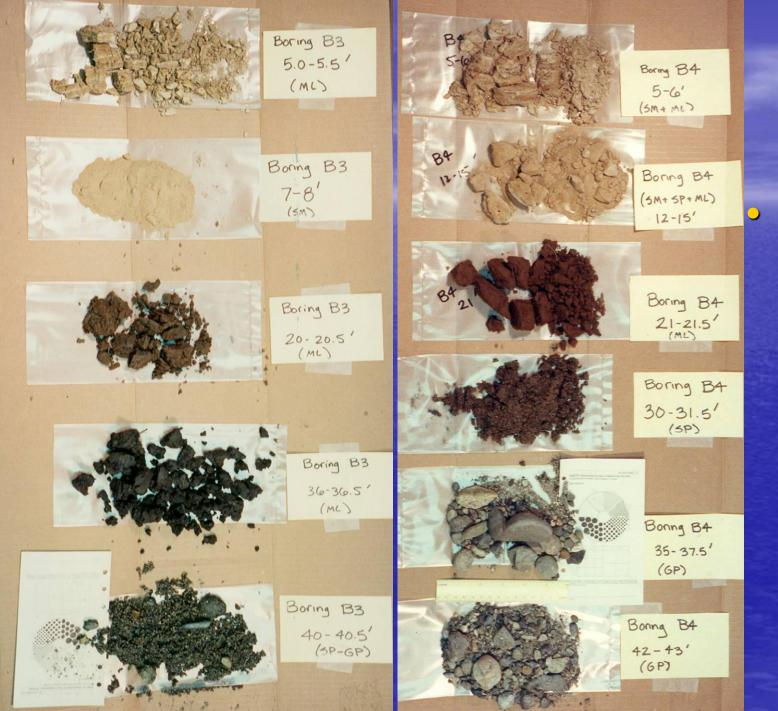
The borings encountered mine slickens over a vibrant paleosol marker, over channel sands, over coarse granitic gravel and cobbles
