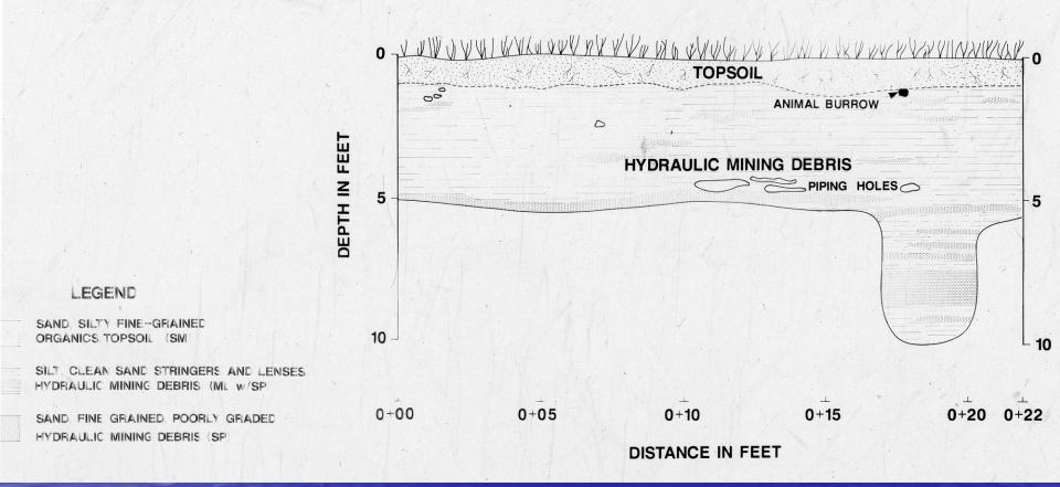
Our site exploration began with a series of trenches along the bounding walls of the channel scoured by the breach outflow. It is important to SEE the stratigraphy in its natural setting BEFORE engaging in subsurface sampling, whenever possible.
