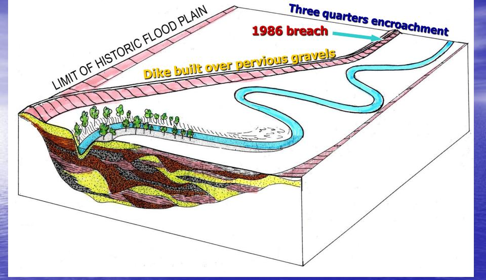
The original protective dike graded in 1873 was along the southern margins of the Yuba River's modern flood plain. The Morrison Grade completed in 1904, and heightened in 1936 and 1940, encroached three quarters of the river's flood plain, as depicted here. Site Characterization should also consider what *natural events* or *man-caused activities* could alter the natural recharge within the prehistoric flood plain
