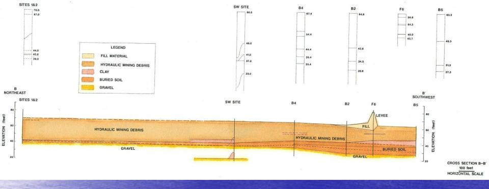
Section B-B' extends from the breach area northwest, towards the main stem channel of the Yuba River.
