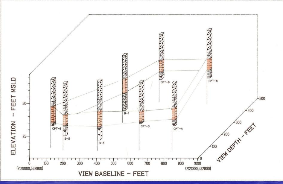
Fence diagrams are useful for assessing threedimensional aspects of the stratigraphy, which are characteristic features of low gradient river channels.
