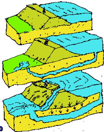
The precise mode of failure remained a major mystery. Eyewitness accounts described a catastrophic landslide-style failure, not the conventional piping style failure we all assume when analyzing earthen levees, as shown here. Some observations by our predecessors....
