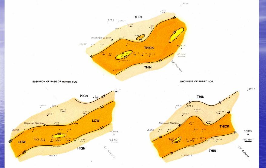
Elevation of buried paleosol; thickness of buried paleosol, and combined thickness of overbank silts and buried paleosol. These units form the *low permeability cap* on the *leaky aquifer* undelying the site.
