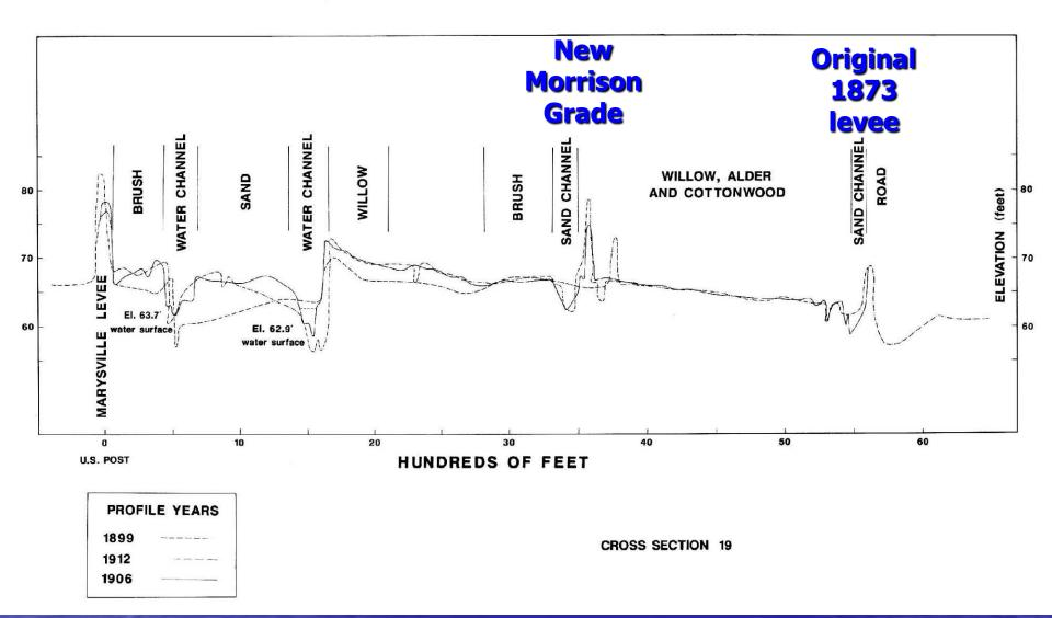
Cross section of the lower Yuba River prepared by the California Debris Commission in 1907. Note gradient of the clogged flood plain, diminishing with increasing distance from the main channel.
