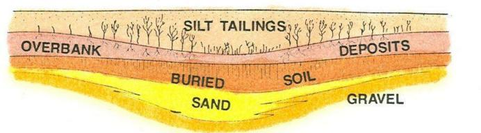
1884 The pre-**1849 flood** plain was inundated by silt tailings from 1862 till at least 1884 Not<u>e axis</u> of swale, beneath breach area
