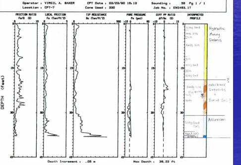
**CPT logs** can be very useful for analyzing *discrete horizons*, *zones of saturation*, and unraveling subsurface stratigraphy; to ascertain the *continuity* of various units. Errant crosshole correlations are a common problem in geotechnical engineering.
