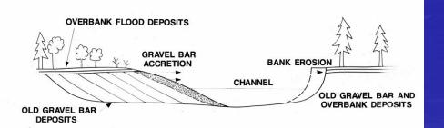
The hydraulic gradient of the Yuba River is about 27X that of the lower Mississippi River, which has, historically, influenced Corps of Engineers design doctrine. The lower Yuba River deposited coarse gravels in *laterally restricted* point bars. Note how these tend to be *discontinuous features*, accreting on the inside bends of the channel, and nonhorizontal These create an *acute* 3D
