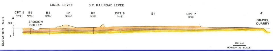
Section A parallels the line of expected seepage and surface flow, from NE to SW. This was extended 1800 ft, to the Speckert Gravel Pit. Note slope of the alluvial materials between the pit and the levee.
