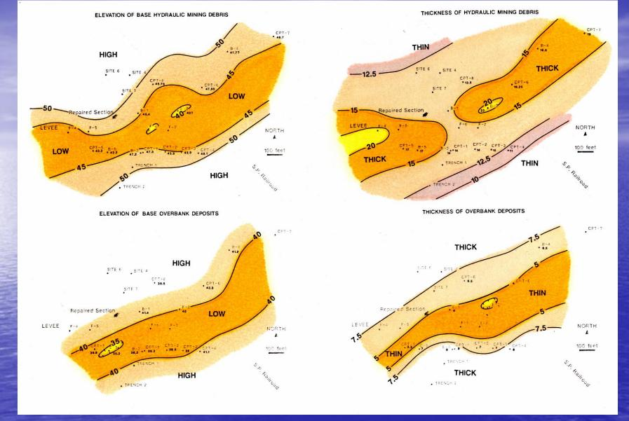
Isopleth and isopach maps of the mine slickens and pre-1862 overbank silt blankets. These suggest a swale, or ephemeral channel, passes through the breach area.
