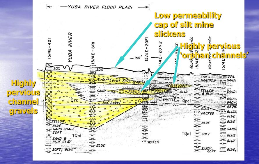
Our interpretation of the well logs along a section through the lower Yuba River, about three miles upstream of its mouth (from Bulletin 6). Water levels were rapidly declining along the south (right) side of the flood plain in the late 1940s. The farmers were drafting water from the channel gravels.
