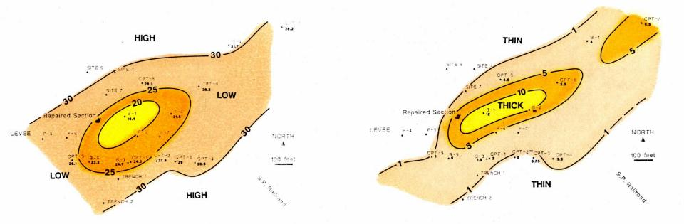
Isopleth and Isopach contours of the Holocene channel sands overlying the late Pleistocene channel gravels.
