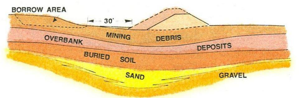
The Morrison Grade was heightened in 1936, using borrow material from the river side of the embankment.
