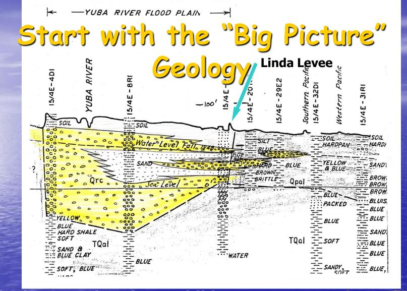
The lower Yuba River exhibits an asymmetric profile, filled with coarse cobbles and sands. Note numerous "orphan channels" extending beyond the southern margins of the modern flood plain.
