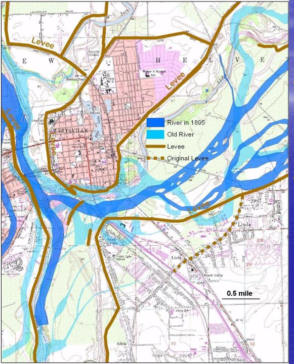
• Taken from first USGS topographic sheet of this area The choked channel has widened considerably, bifurcated, and developed numerous islands and bars.
