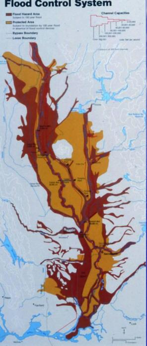
Sacramento Valley Flood Control System Developed by Carl E. Grunsky and approved by the California **Debris Commission/Corps of Engineers in 1913; Constructed** between 1914-60 It employs earthen levees to protect populated areas It conveys excess flood waters through a system of bypass weirs that spill into large basins (shown in dark brown), limited to agricultural usage
