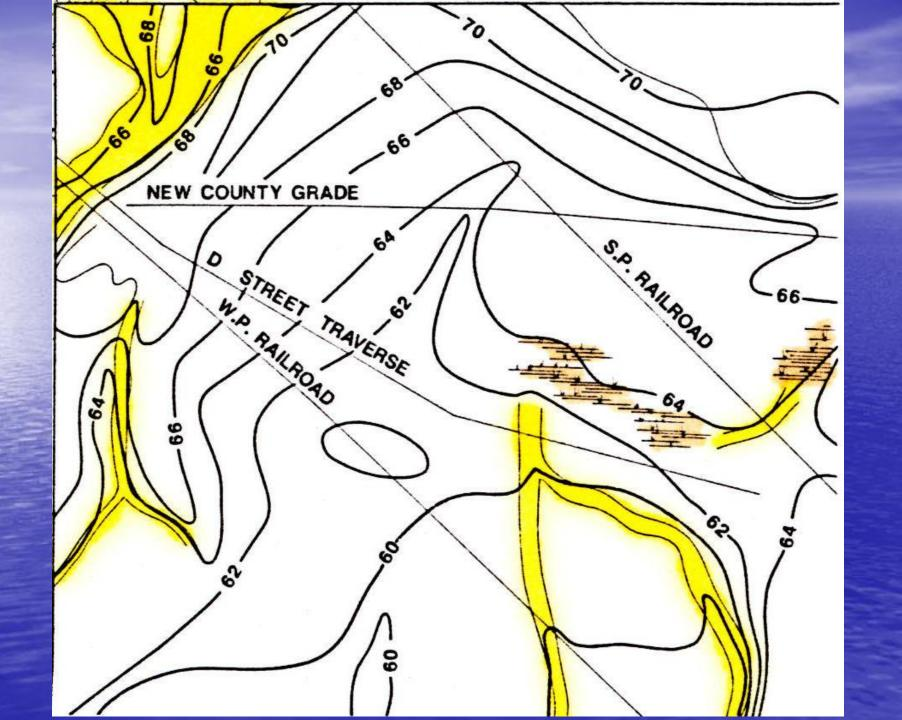
**1907 TOPOGRAPHY Exploration program began with 4 borings along surviving levee crest, followed by 5 conventional auger borings, 7 CPT soundings, two trenches, augmented by 3 borings by others.**
