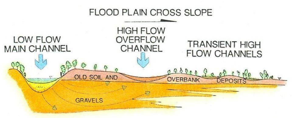
Like any overbank silt, the hydraulic mine slickens deposited after 1862 tended to be thickest near the main stem channels, diminishing outward. Overflow channels would periodically carve material off, reducing thickness of the slickens and overbank silts along those ephemeral channels.
