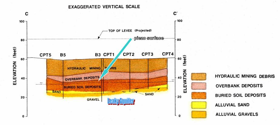
Pore pressures emanating from the cobble gravels extend into the low permeability paleosol cap. As soon as flood waters filled the Speckert gravel pit, that pressure head would have acted on the leaky aquifer, engendering considerable uplift ACTUAL VERTICAL SCALE Full-blown liquefaction-induced 'softening' versus pore pressureinduced destabilization
