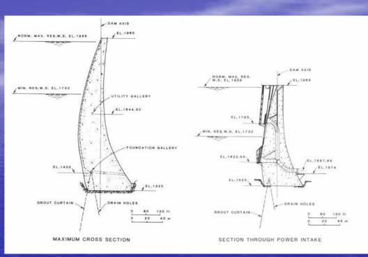
The largest double curvature concrete arch dam in the USA was completed along the North Fork of the Yuba River in November 1969, replacing an older dam
