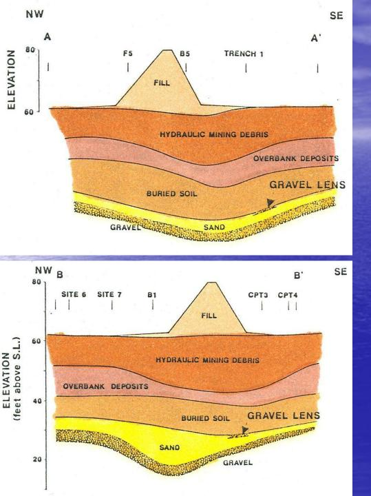
Sections through breach area Sections A-A' and **B-B' were cut** perpendicular to the 1907 swale, normal to the historic direction of flow of the Yuba River. Note axes of previous swales in succeeding deeper units.
