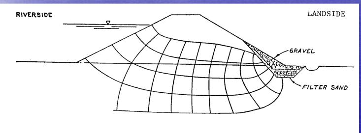
c. Pervious toe combined with partially penetrating toe trencn
