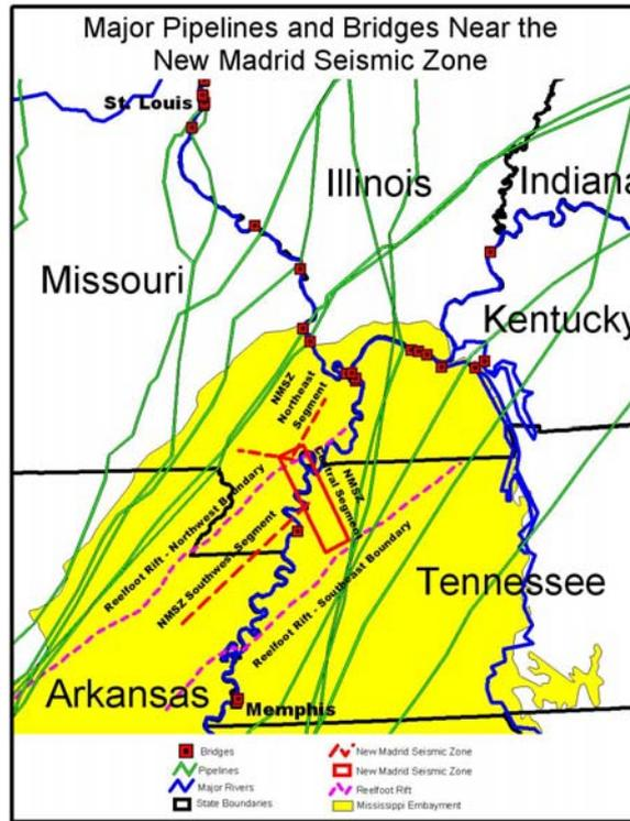
**Fig. 7. Major pipelines (in green) and highway bridges (red squares) in the New Madrid Seismic Zone, compiled by David Hoffman at Missouri S&T. The faults are shown as dashed red lines, while the approximate limits of the underlying Reelfoot Rift are delineated by dashed pink lines.**
