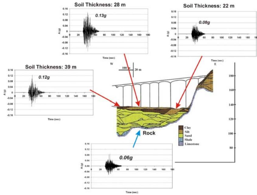
Fig 3. Effect of soil thickness on peak ground acceleration from a Magnitude 6.8 earthquake striking the Creve Cour Bridge on the southern bank of the Missouri River about 110 km from a quake centered in south central Illinois.
