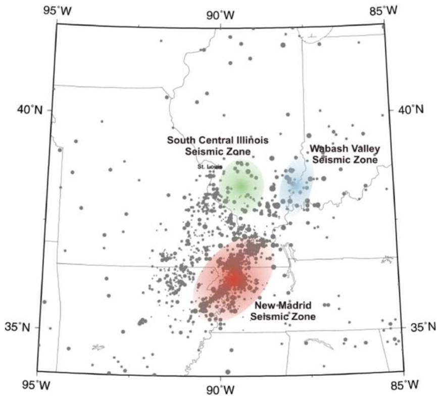
**Fig. 1. Seismic source zones in the central United States. South Central Illinois is an area of diffuse seismicity which is not well documented or yet understood, because it is covered by glacial outwash.**
