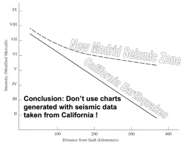
**Fig. 2. Contrast between damping of shaking intensity with distance from seismic sources in California and the Midwestern US (taken from Bolt, 2003). Most damping models prior to 2000 were biased by data from California earthquakes.**
