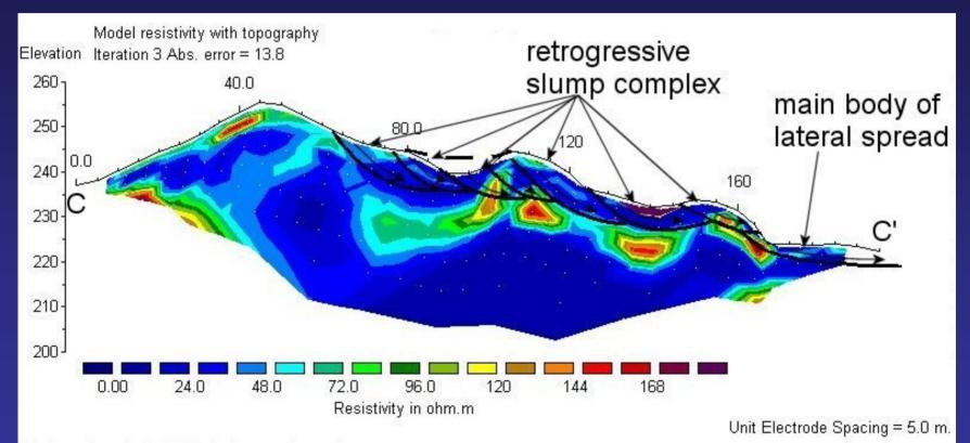
Horizontal scale is 18.72 pixels per unit spacing Vertical exaggeration in model section display = 1.00 First electrode is located at 0.0 m. Last electrode is located at 195.0 m.
